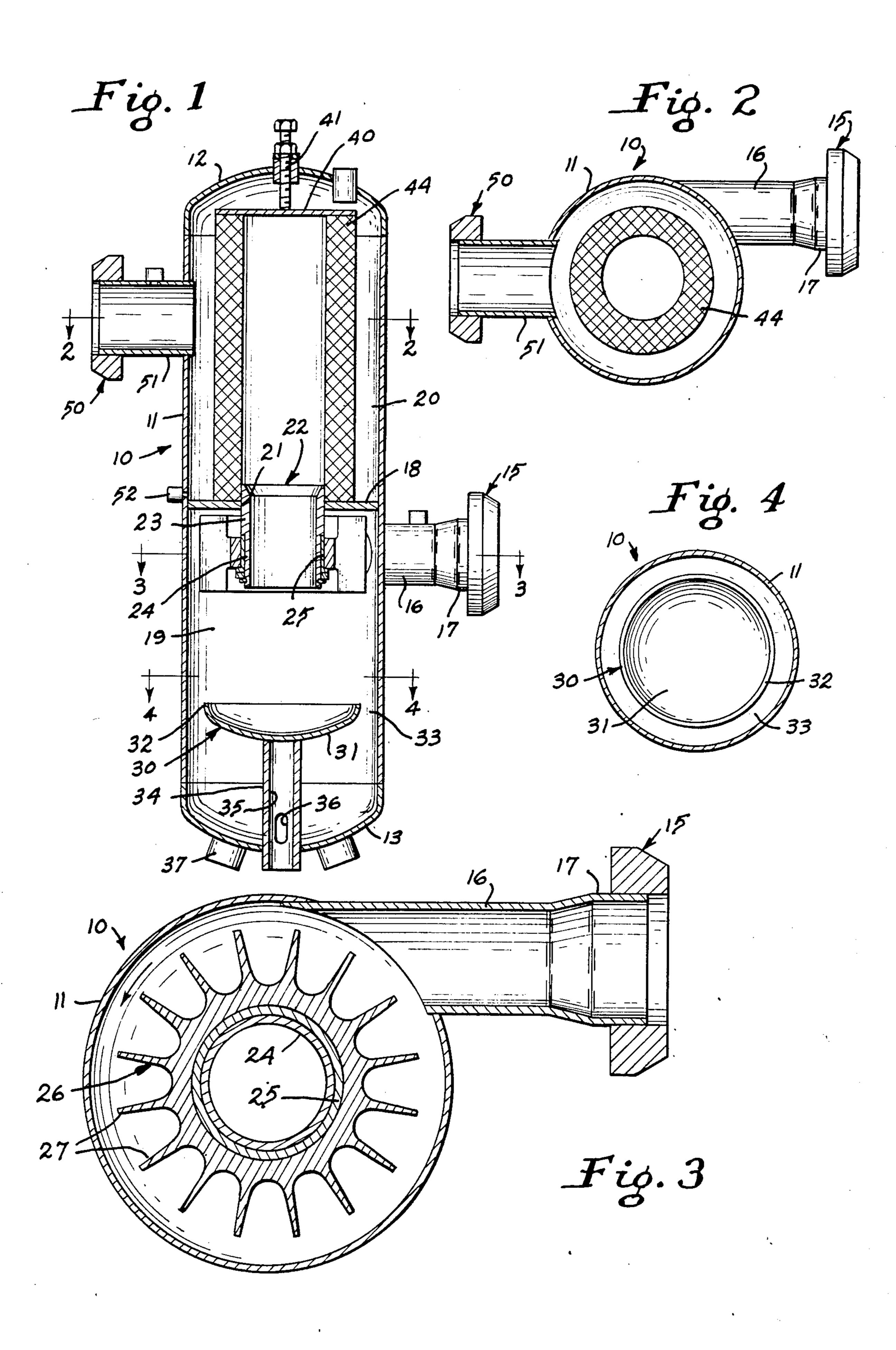
impinges, the oil then draining downwardly from the disk and the vapor being deflected upwardly through a central outlet member.
