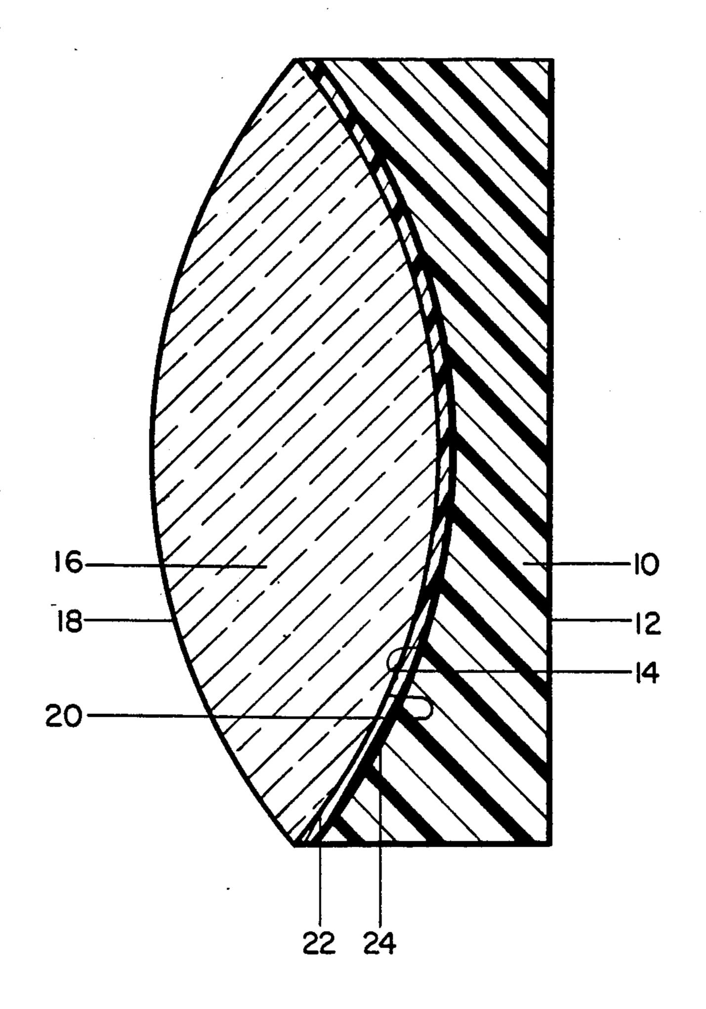
the lens elements, in combination with a primer coating of an aliphatic polyurethane on the optical surface of at least the plastic lens element.
