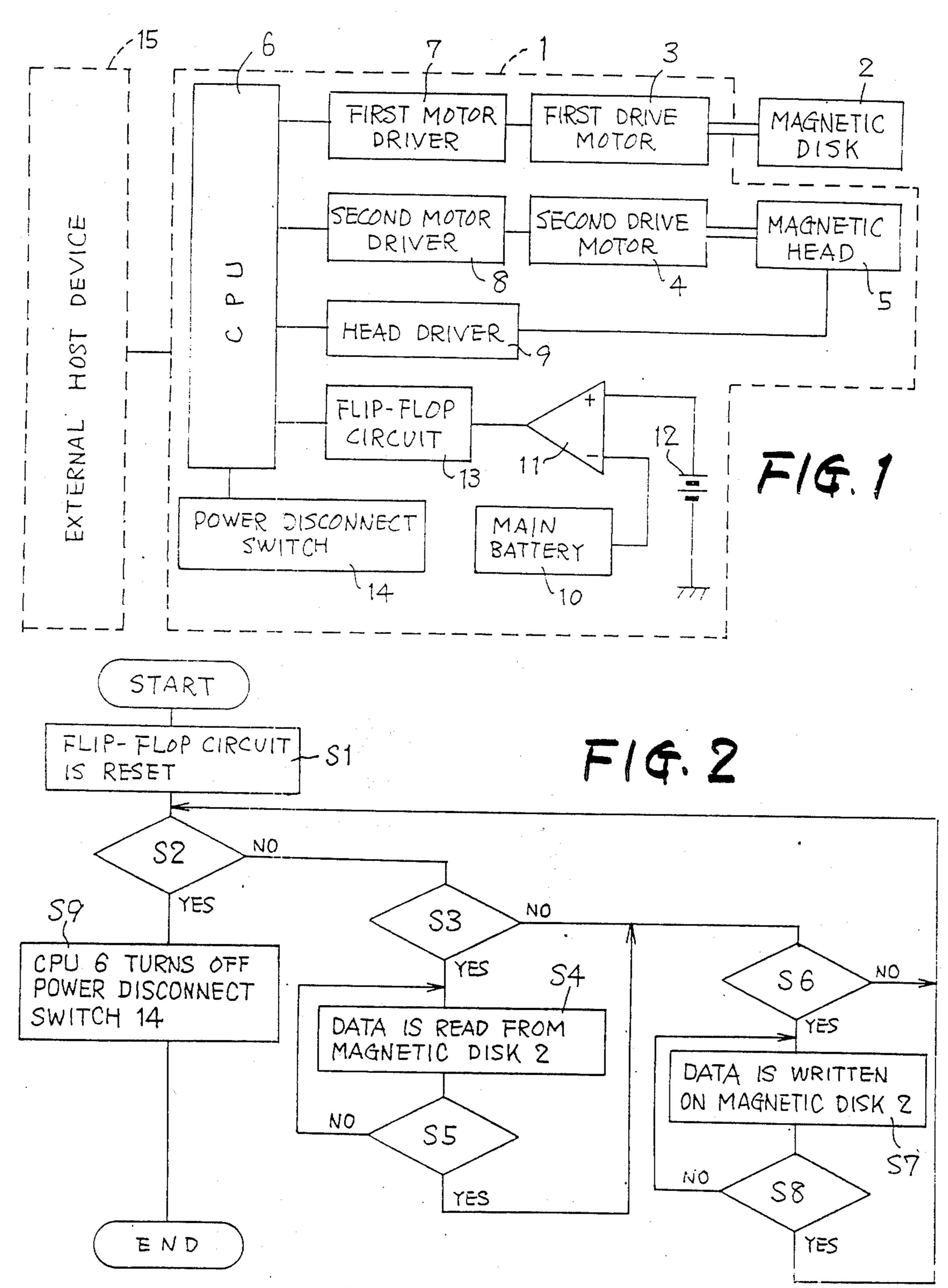
S2: CPU 6 CHECKS IF A VOLTAGE-DROP SIGNAL IS PRESENT
