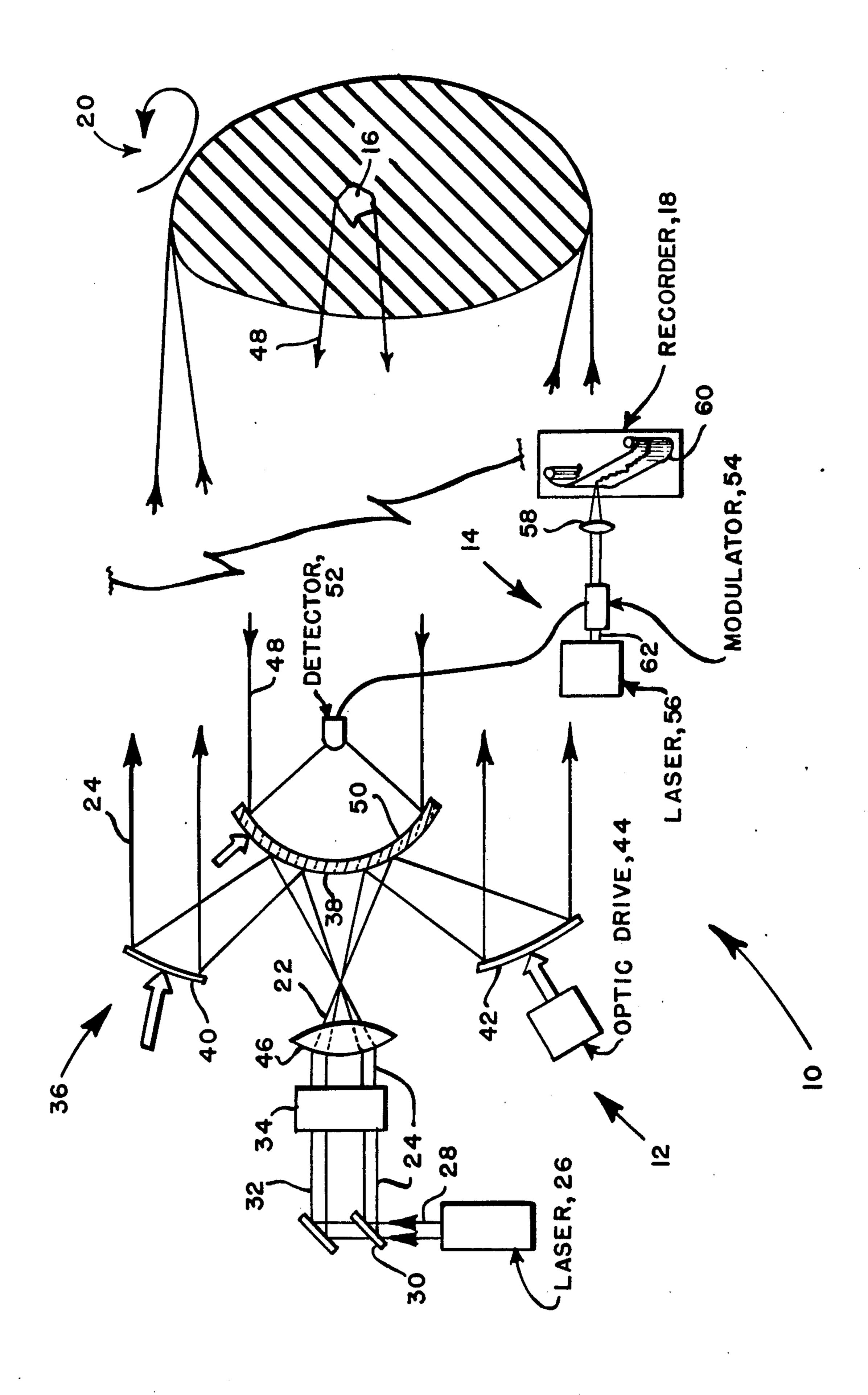
SYNTHETIC APERTURE LASER RADAR
