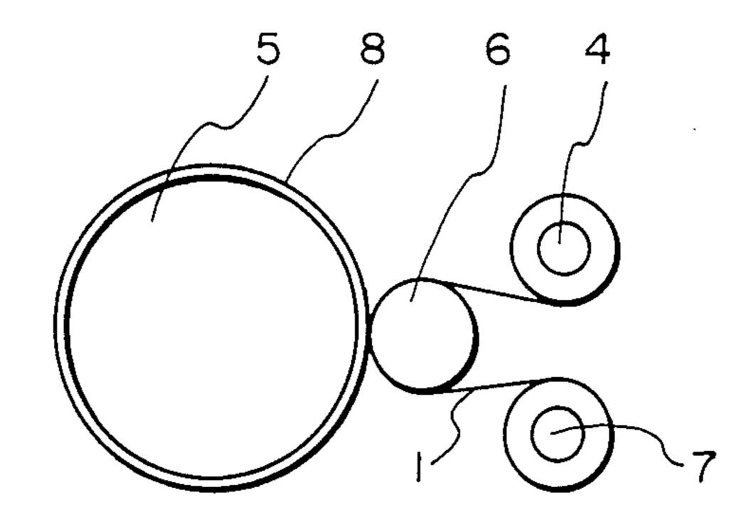
CLEANING WEB FOR FIXING ROLLS ON COPY **MACHINES**
