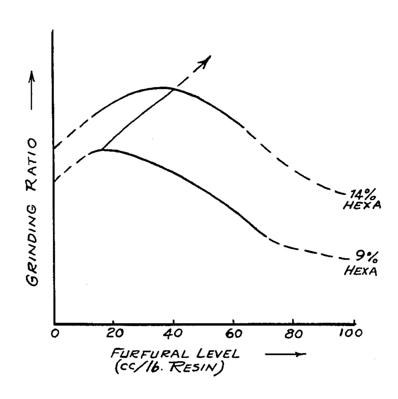
SCHEMATIC DIAGRAM OF GRINDING RATIO VS FURFURAL CONTENT AT VARIOUS HEXA LEVELS
