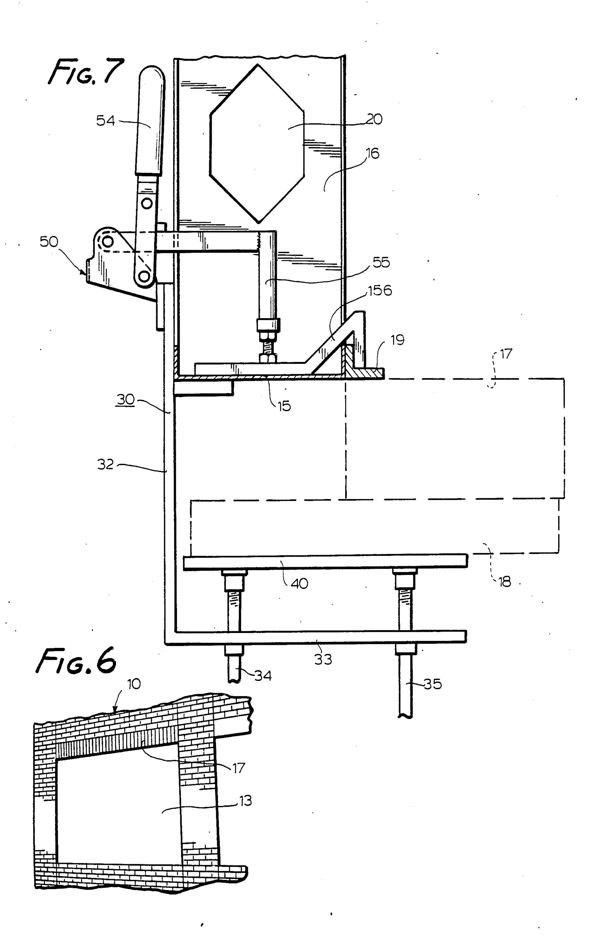
APPARATUS AND METHOD OF SHORING MASONRY, STONE, CONCRETE AND OTHER MATERIALS OVER OPENINGS IN BUILDINGS
