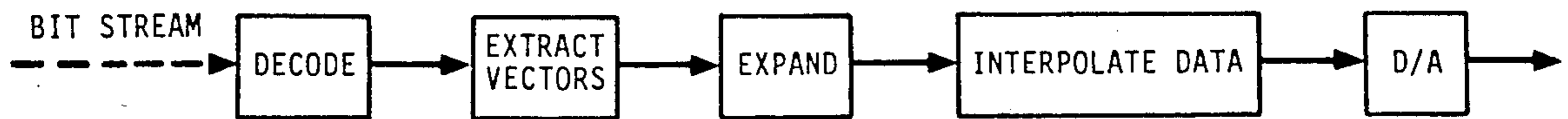
FIGURE 25 BLOCK DIAGRAM OF RECEIVER
