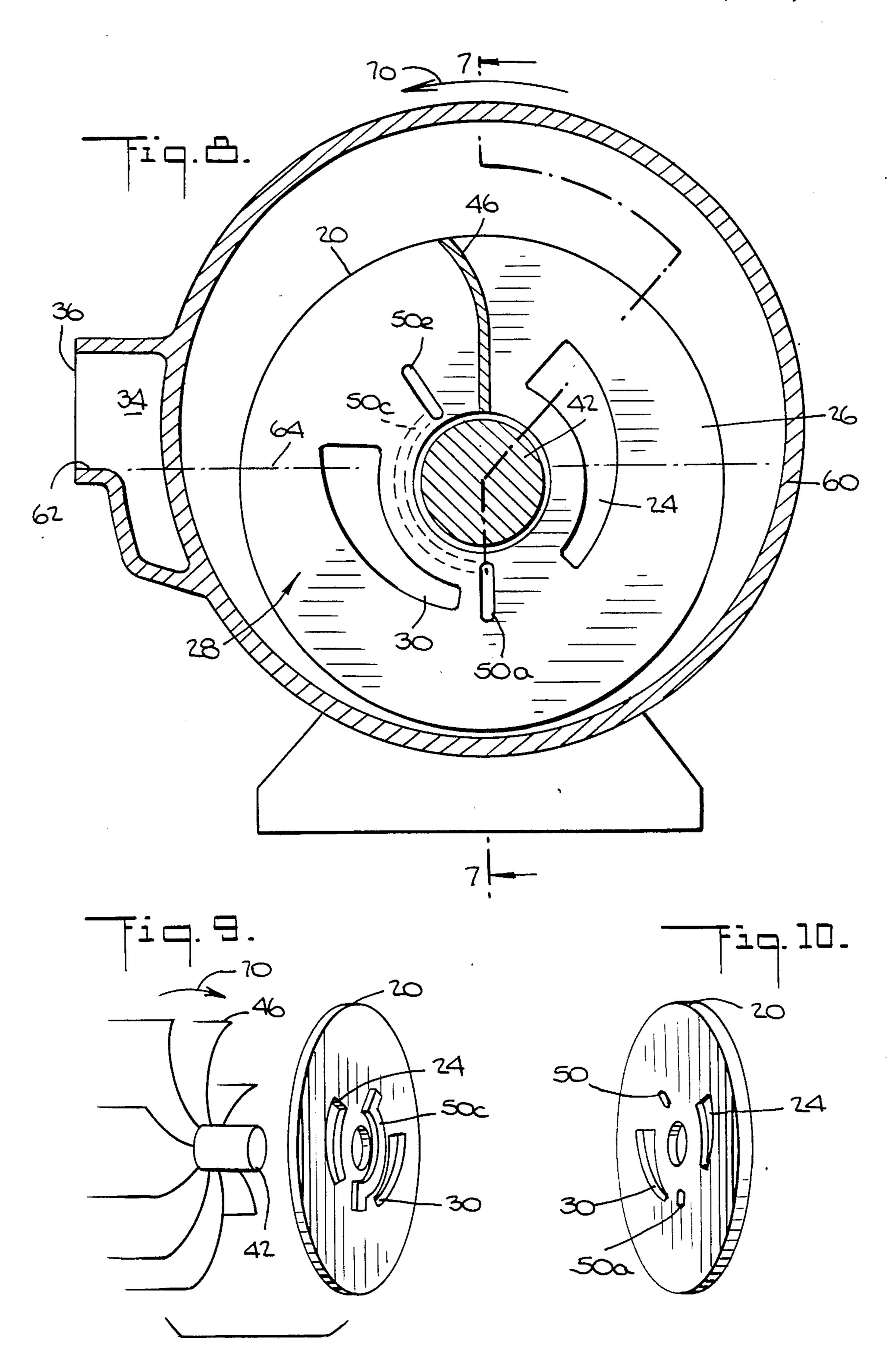
SELF-PRIMING LIQUID RING PUMP METHODS AND APPARATUS
