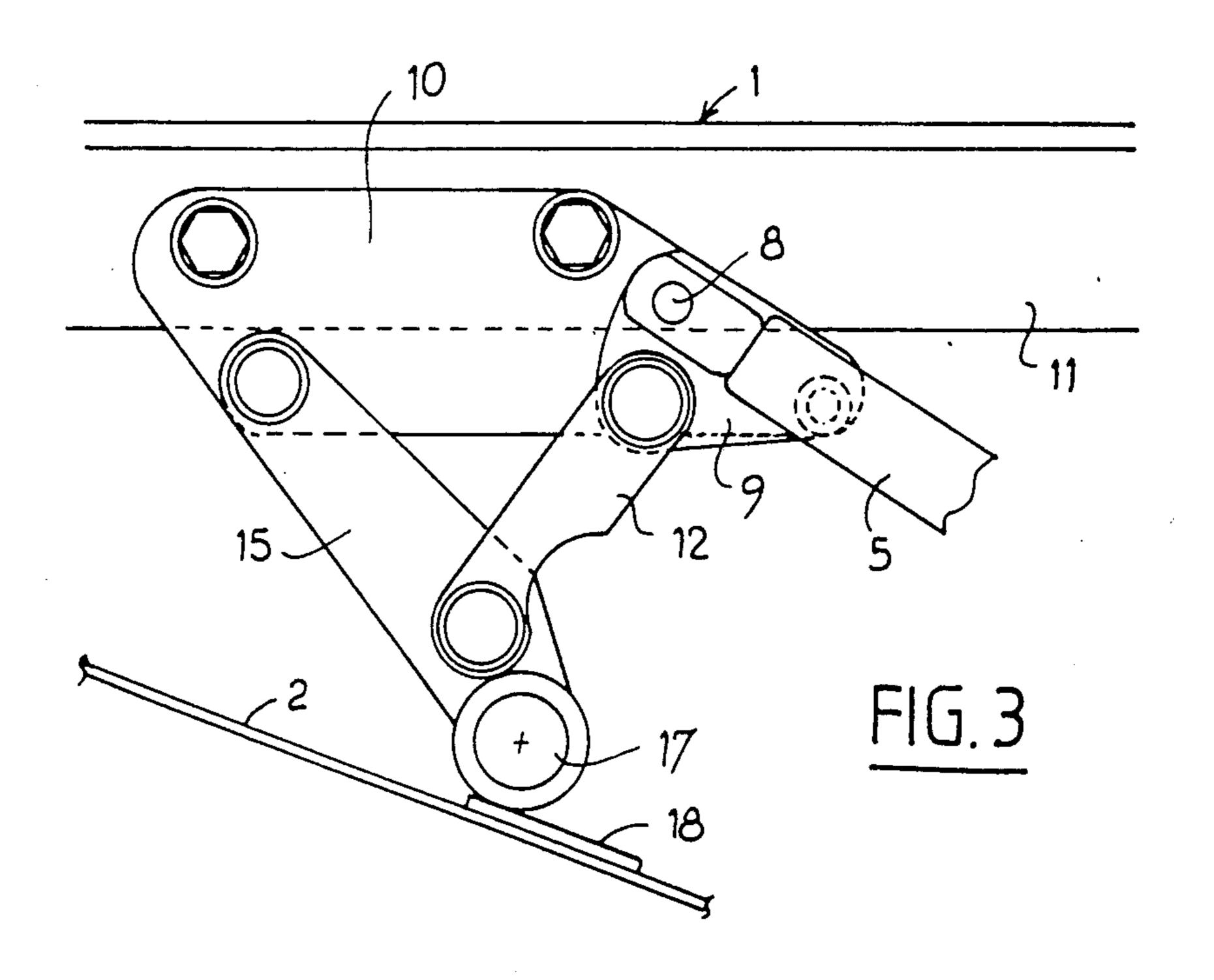
COUNTERBALANCING DEVICE FOR HATCHBACK LID ON A ROAD VEHICLE
