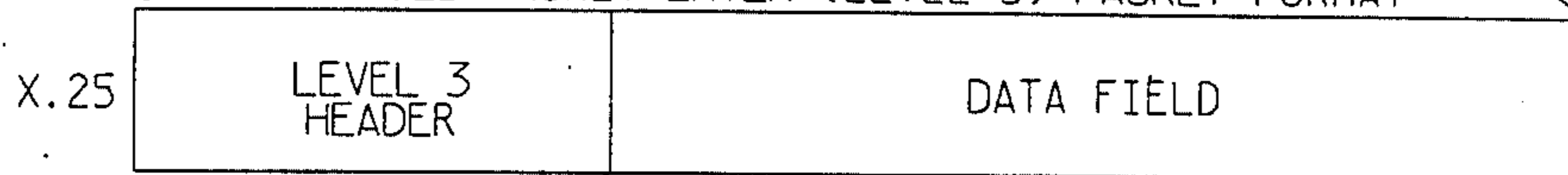
X.25 PACKET LAYER (LEVEL 3) PACKET FORMAT
