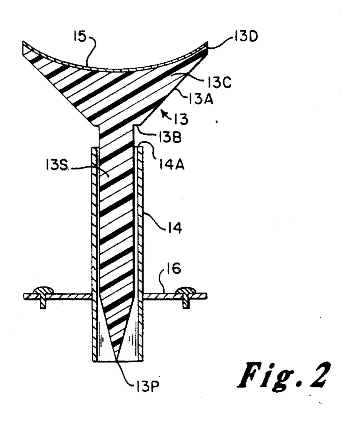
ing material 15 at the outside concave surface. A base 16 is screwed to appropriate supports in conventional manner, and there is a conventional feed for coupling the inside end of the dielectric waveguide 13 to waveguide coupled to transmitting and/or receiving equipment.
