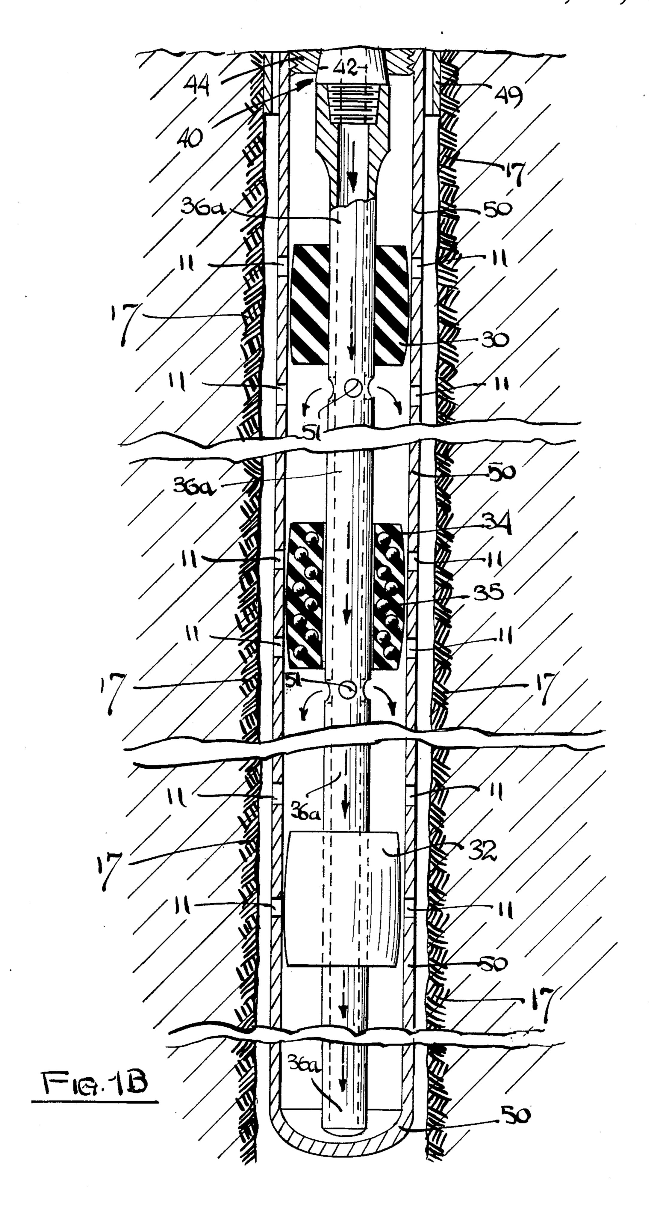
METHOD FOR SONICALLY LOOSENING OIL WELL LINER ENVIRONMENTS
