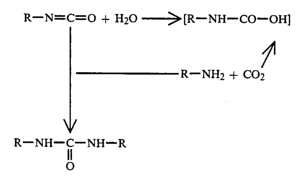
Moisture hardening can lead to undesired bubble 45 formation, while the hardening speed depends greatly on the humidity present in the air and is therefore difficult to control. The hardening takes place very slowly from the outermost layers inward, and not simultaneously in the whole mass, as in two-component prod-50 ucts.
