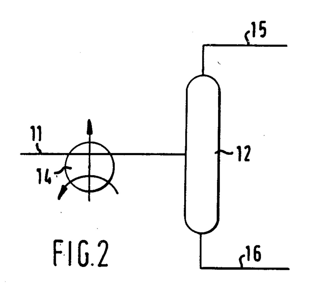
separator connected to the discharge line and provided with an upper discharge line and a lower discharge line.
