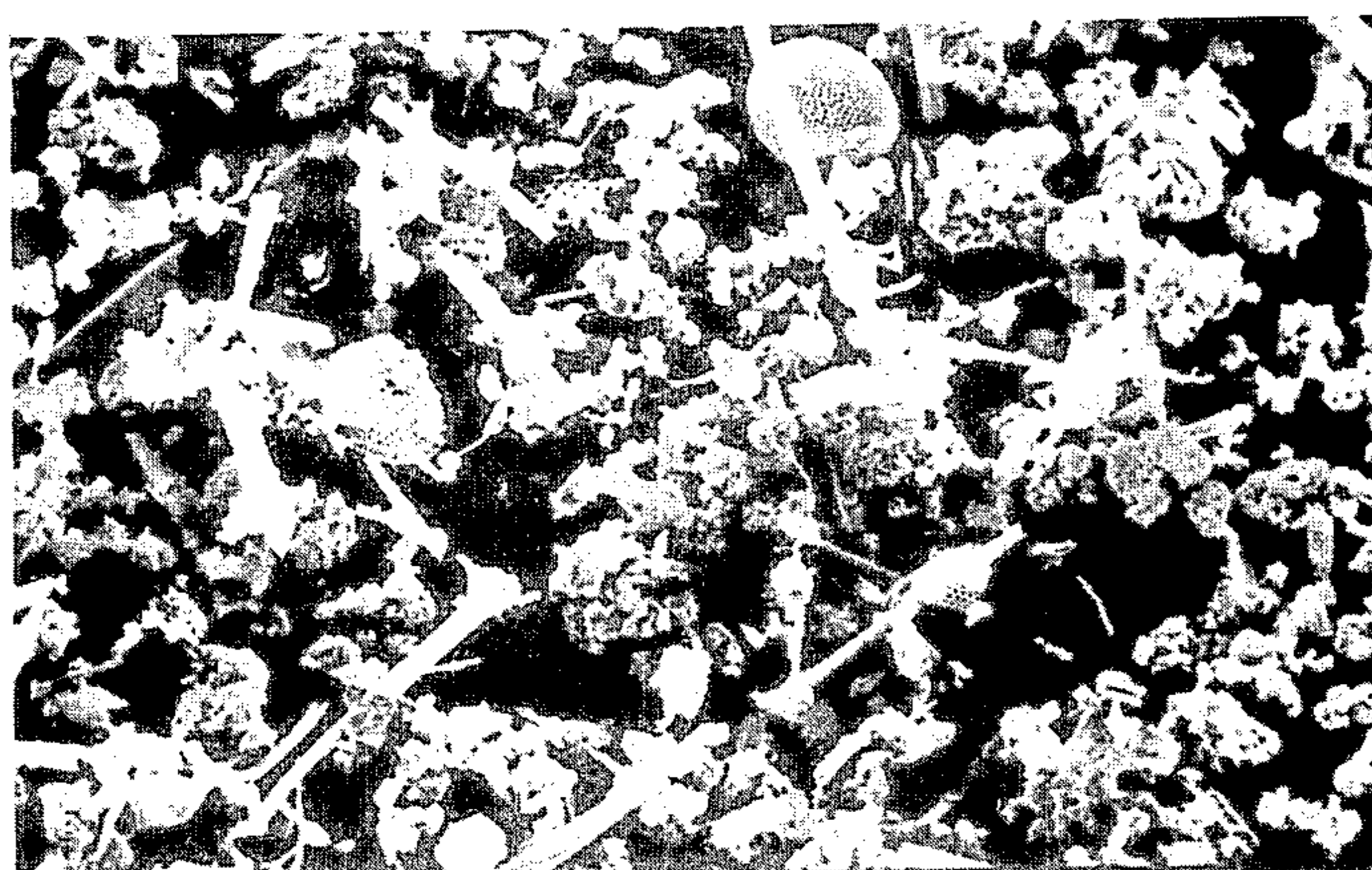
FIG. 2 Electron micrograph Guhr catalyst 100 r.p.m. magnification 500 x (1mm - 2um)
