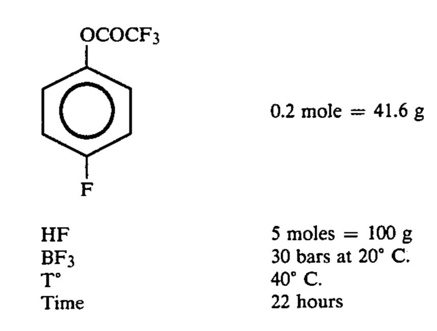
After treatment, analyses by a combination of gas phase chromatography and mass spectrometry show the presence of 4-fluoropentafluoroethoxybenzene.
