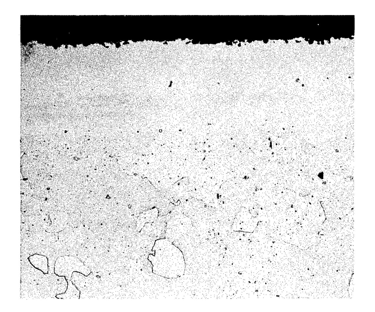
DIFFUSION TREATED HOT-DIP ALUMINUM COATED STEEL
