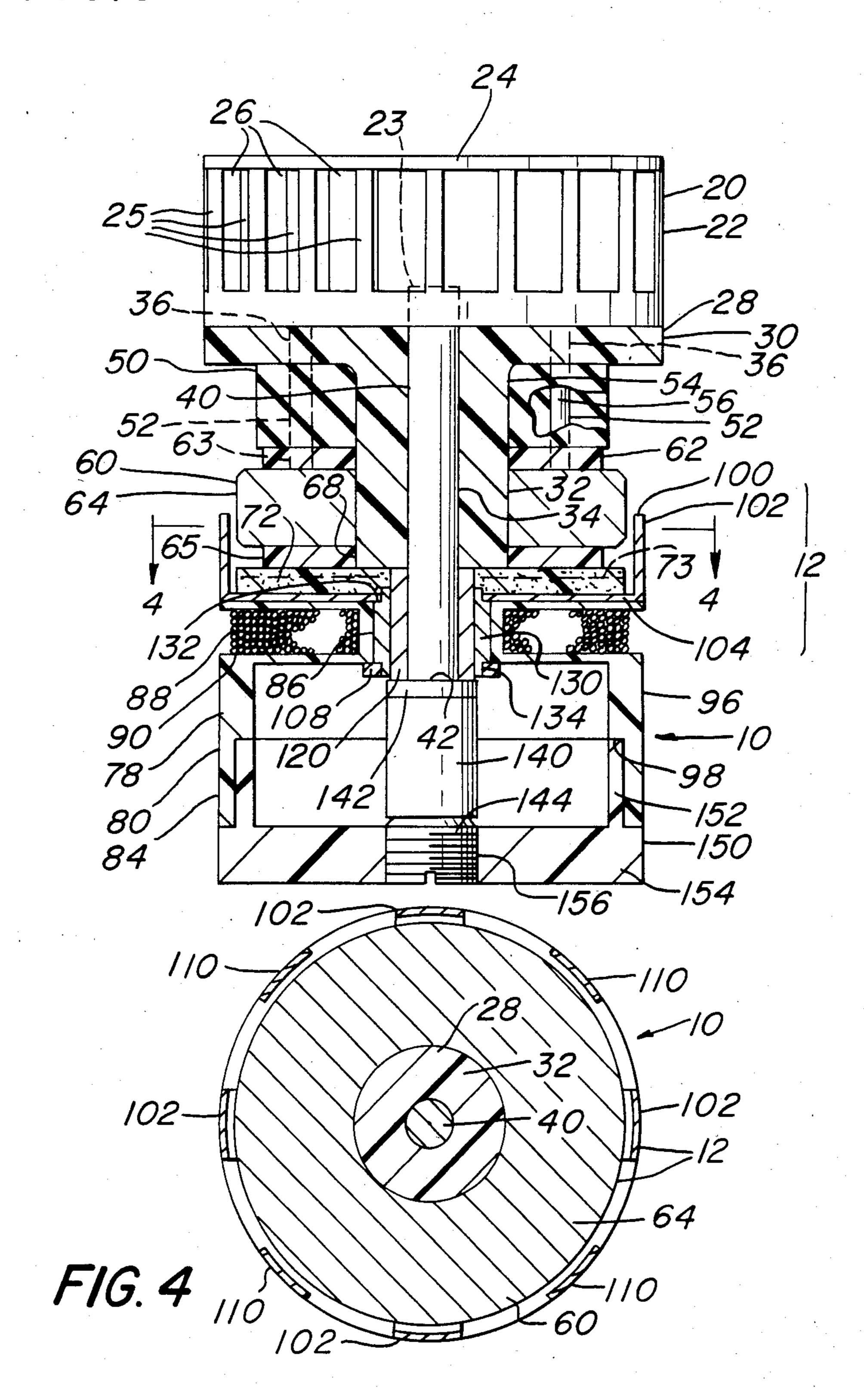
ELECTRIC GENERATOR ASSEMBLY FOR A PROJECTILE
