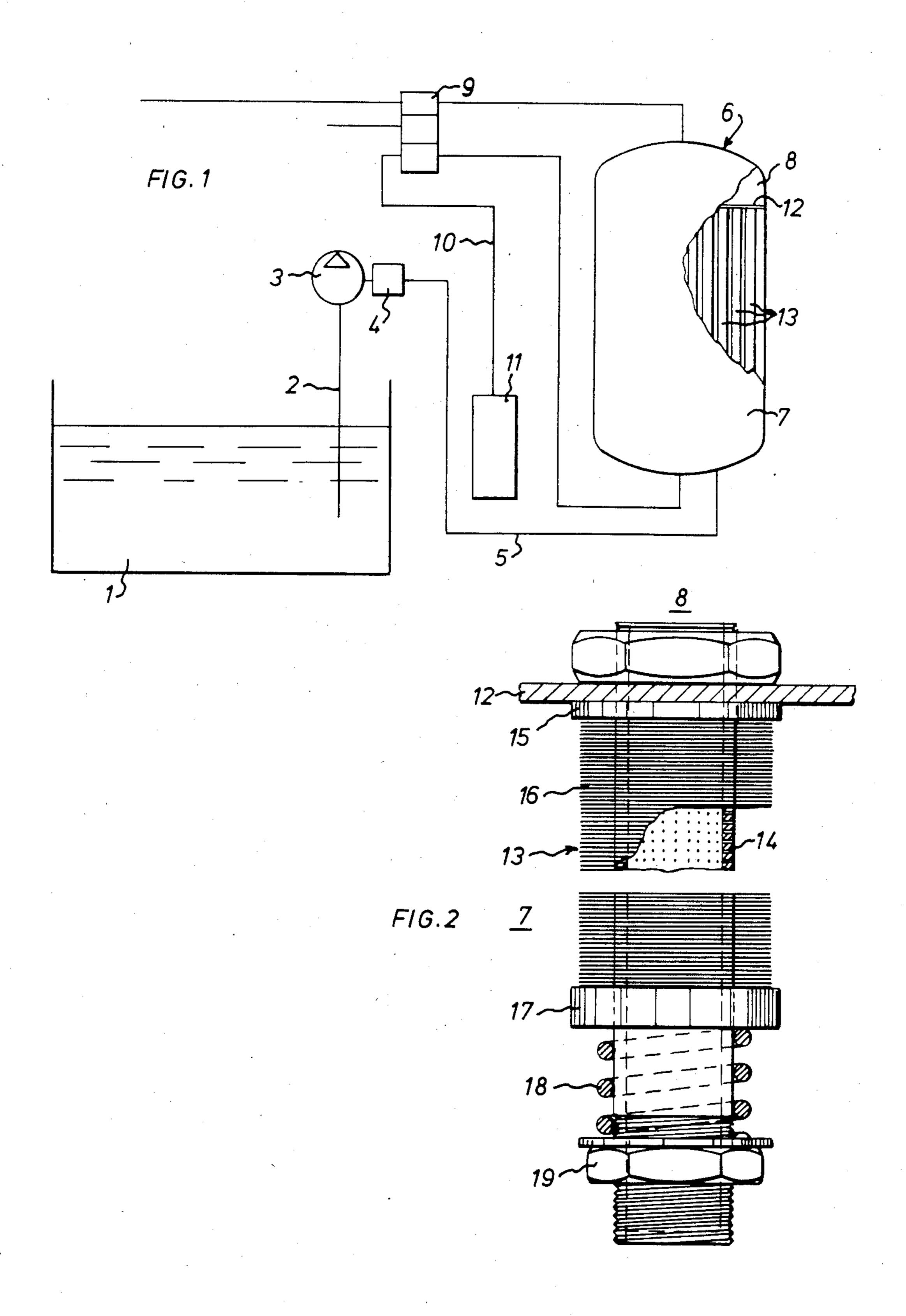
METHOD AND INSTALLATION OF FILTRATION WITH COMPRESSIBLE DISCS
