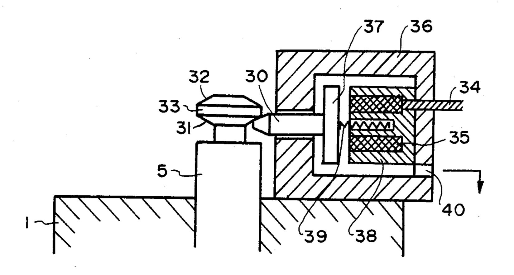
During operation, all that the actuating mechanism need do is to retain the valve in each of the two end positions. That is, the actuating mechanism becomes a passive retaining element which ceases to be "responsible" for moving the valve.
