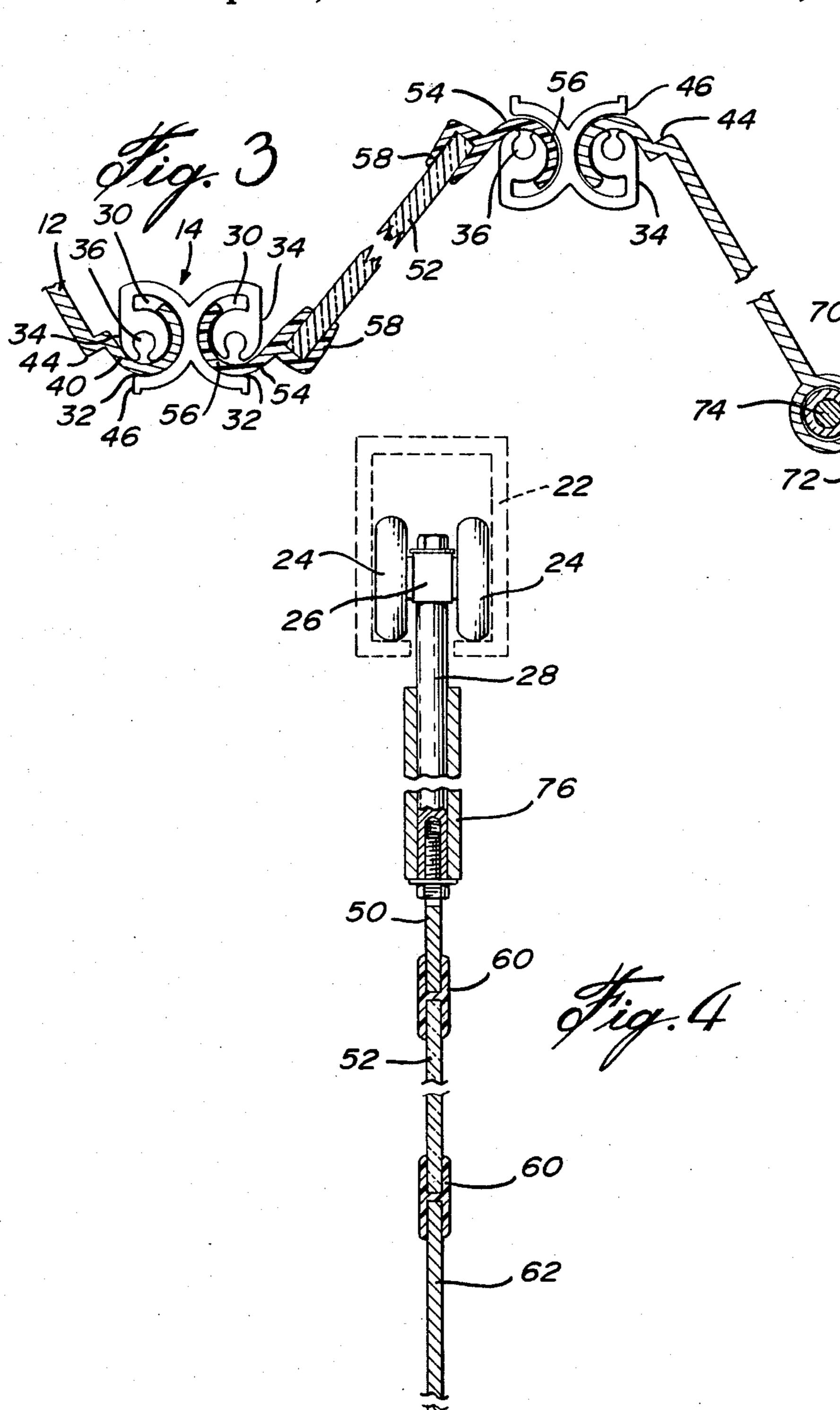
The present invention relates to a folding closure or door having a series of vertical strip panels vertically 5 hinged together and supported by rollers running in a top track.
