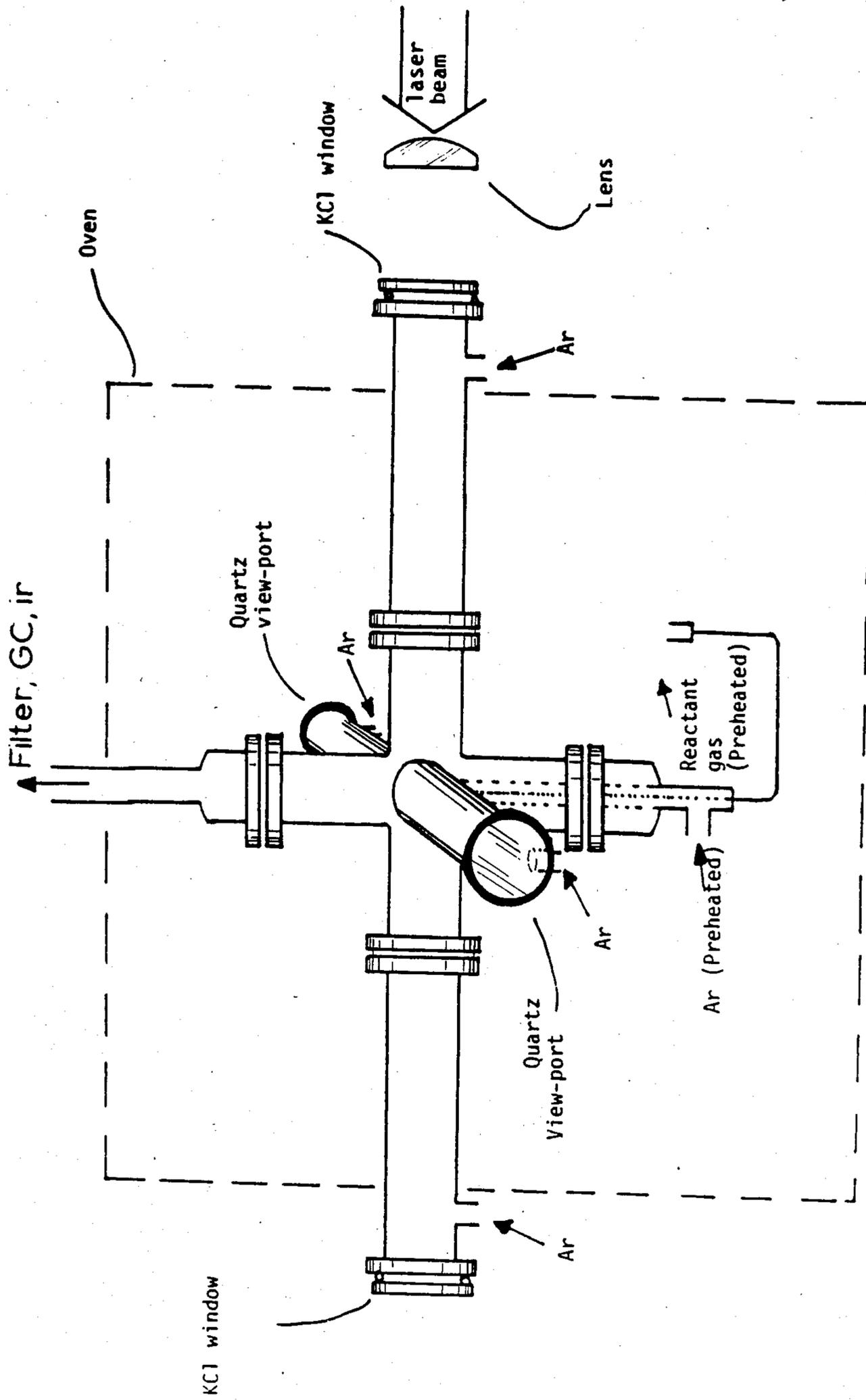
Figure 1. Laser Synthesis Reactor
