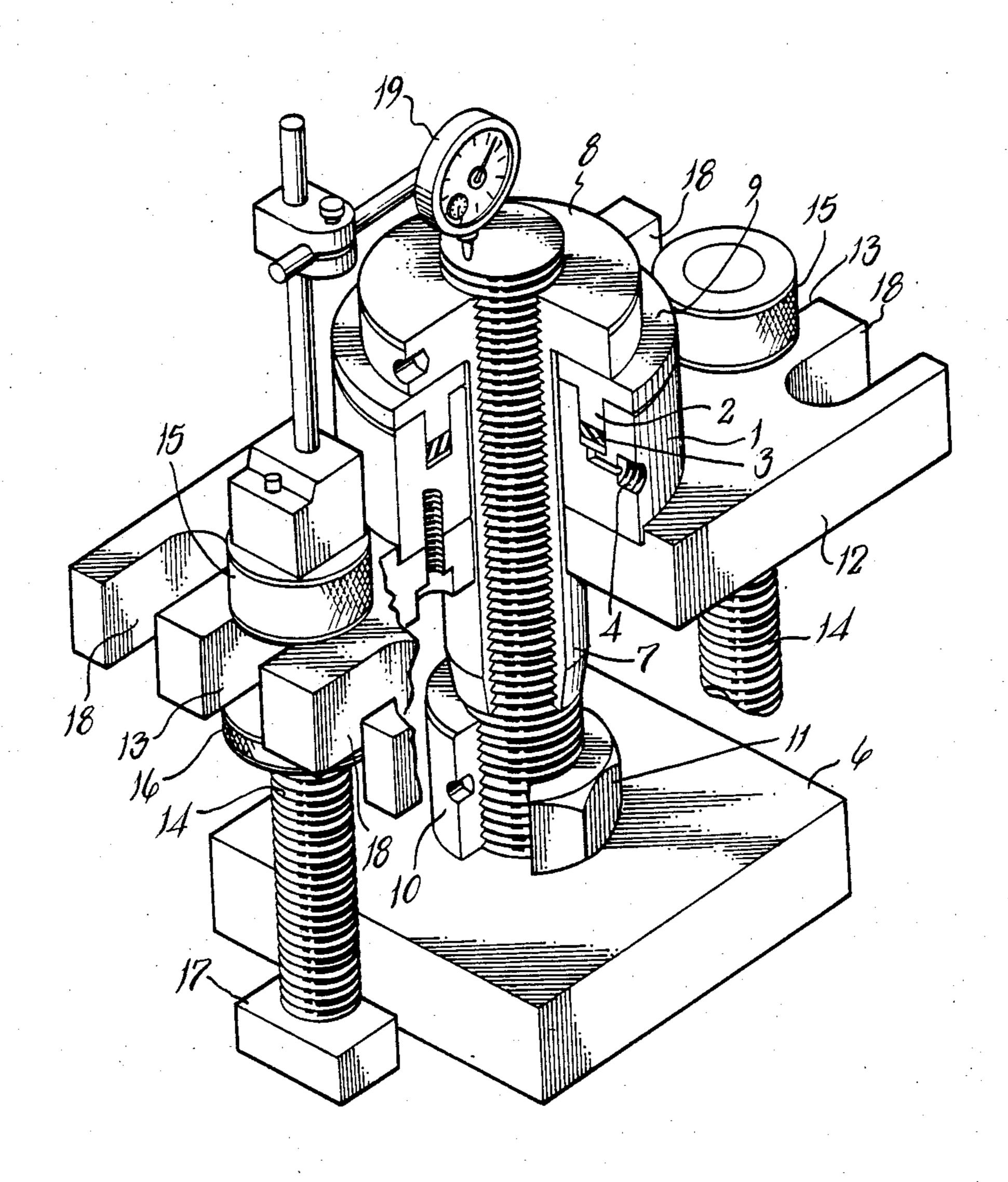
where access for a conventional bridge piece is difficult, or impossible. Hitherto it has been necessary to make special asymmetrically shaped bridge pieces for some jobs which can now be handled much more easily with the tensioner of this invention.
