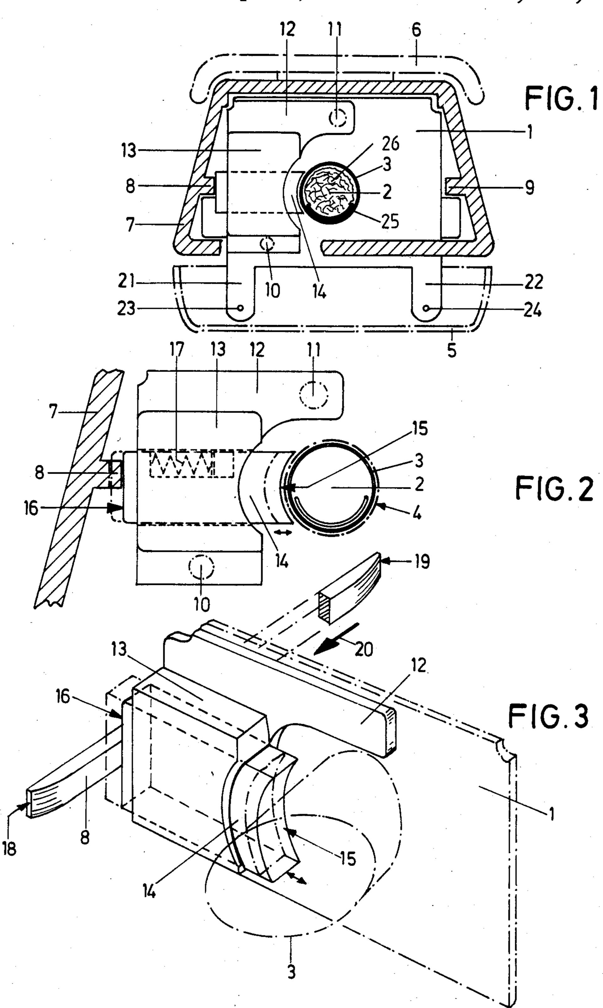
geous in a further embodiment of the invention for the control ledge to be embodied in such a manner, for instance being beveled, in its terminal-position areas that no displacement of the clamping element is possible when it is in one of these terminal positions, or that the clamping element is retracted from the cigarette tube by
