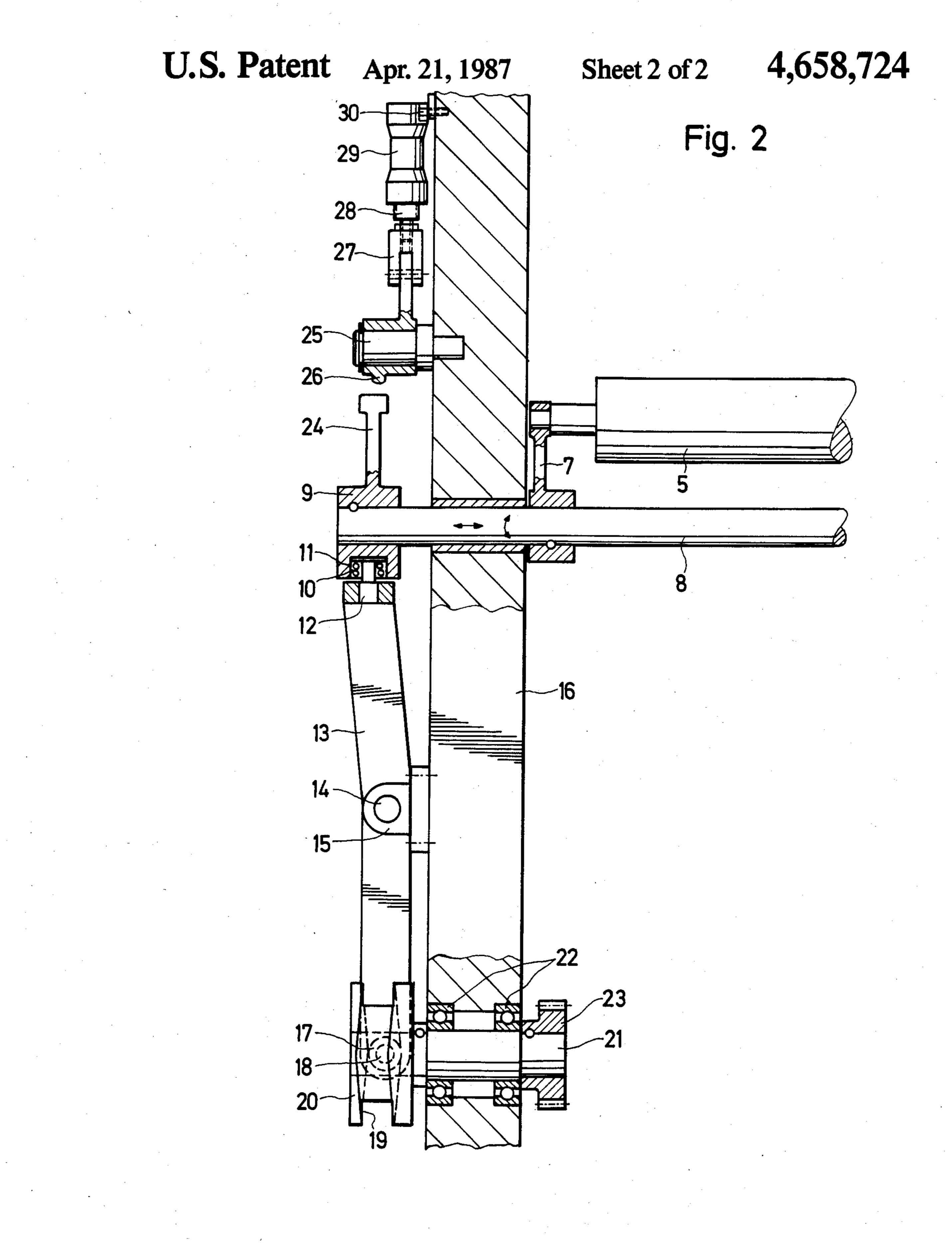
DEVICE FOR TRANSFERRING INK TO AN INKING UNIT OF A PRINTING MACHINE
