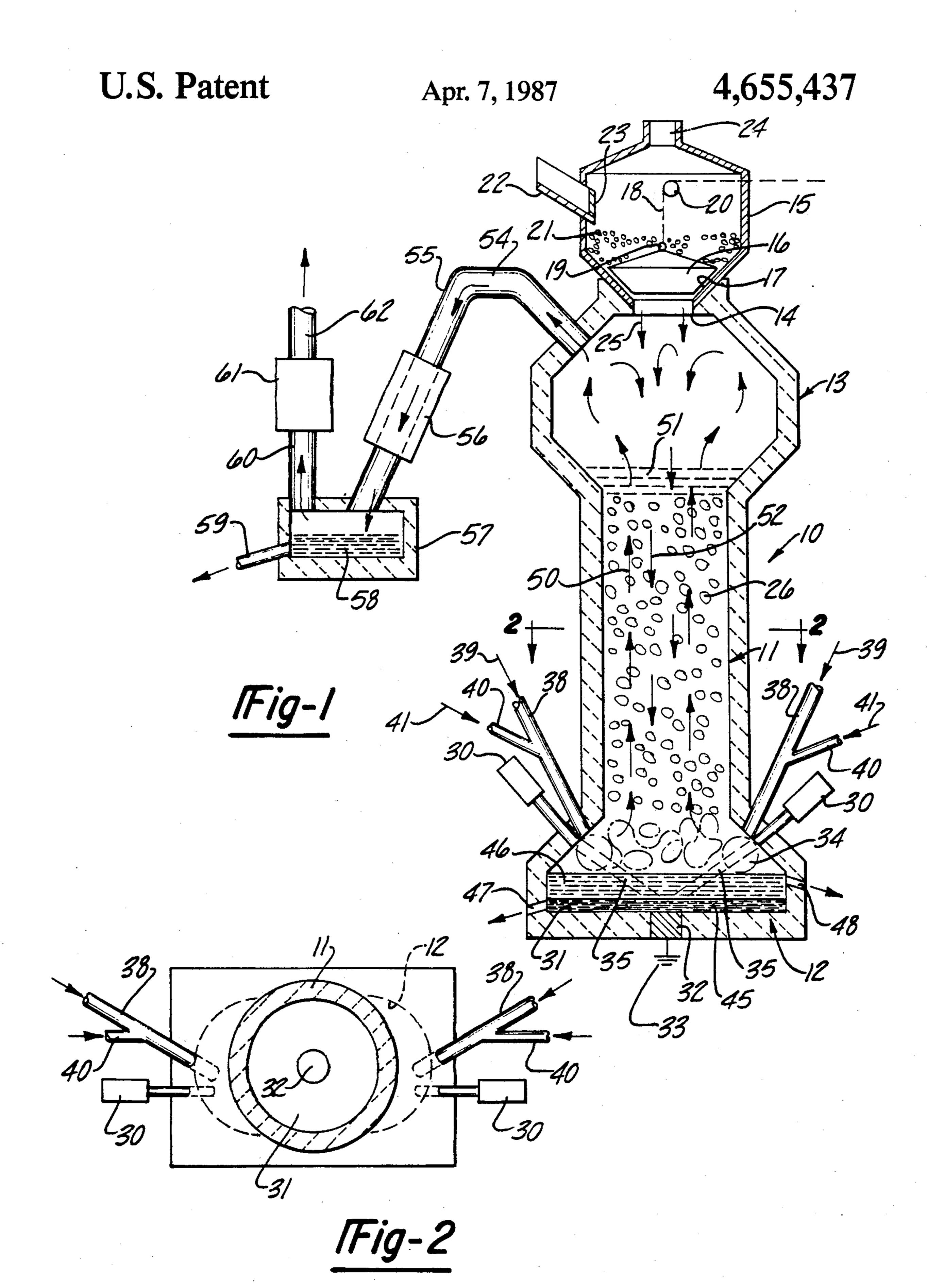
APPARATUS FOR SIMULTANEOUSLY SEPARATING VOLATILE AND NON-VOLATILE METALS
