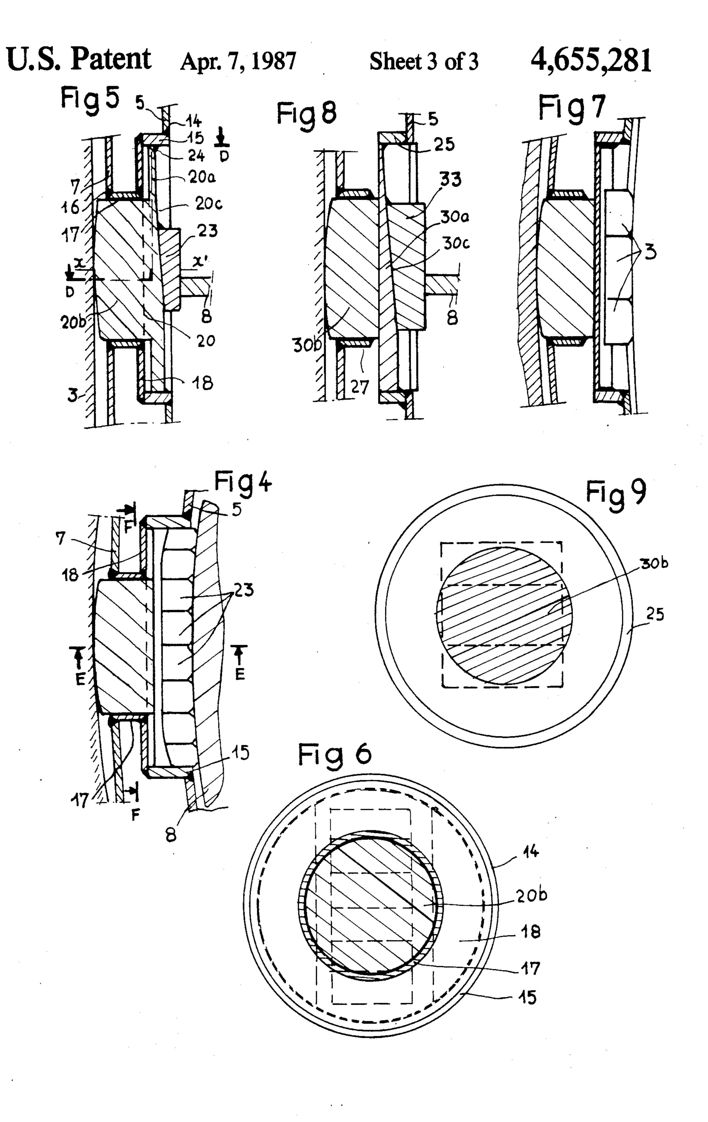
HEAT EXCHANGER INCORPORATING A TUBE BUNDLE ARRANGED IN A CYLINDRICAL BUNDLE CASING HELD RADIALLY INSIDE AN OUTER CYLINDRICAL CASING
