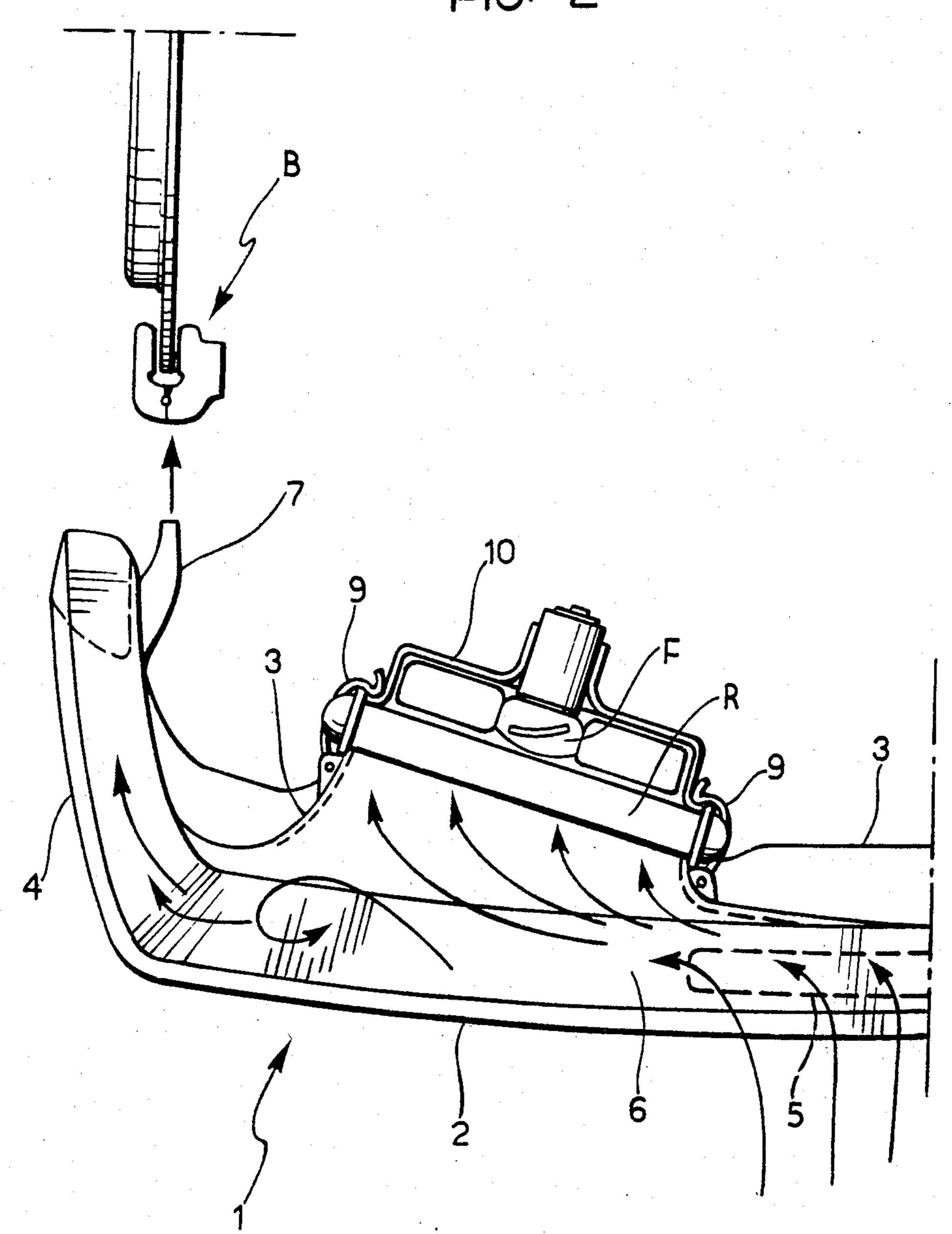
partment and with the ends 4 bent towards the rear wheels of the vehicle.
