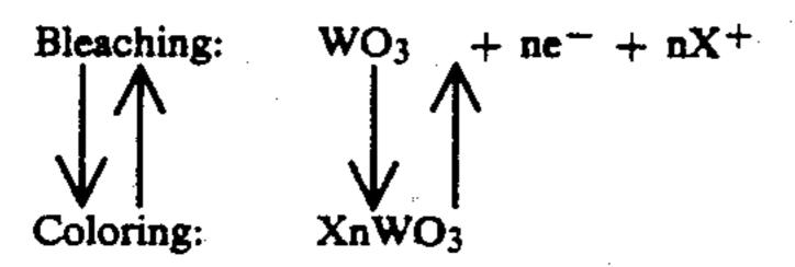
Protons (H+) are used as the cations (X+) since the proton has a small ion radius and high mobility. The cations need not always be in the state of cations. More specifically, it is essential to generate cations when a 40 voltage is applied across the electrochromic device. For protons, water is used as a cation source. Water is decomposed upon application of a voltage thereto in accordance with the following general reaction:
