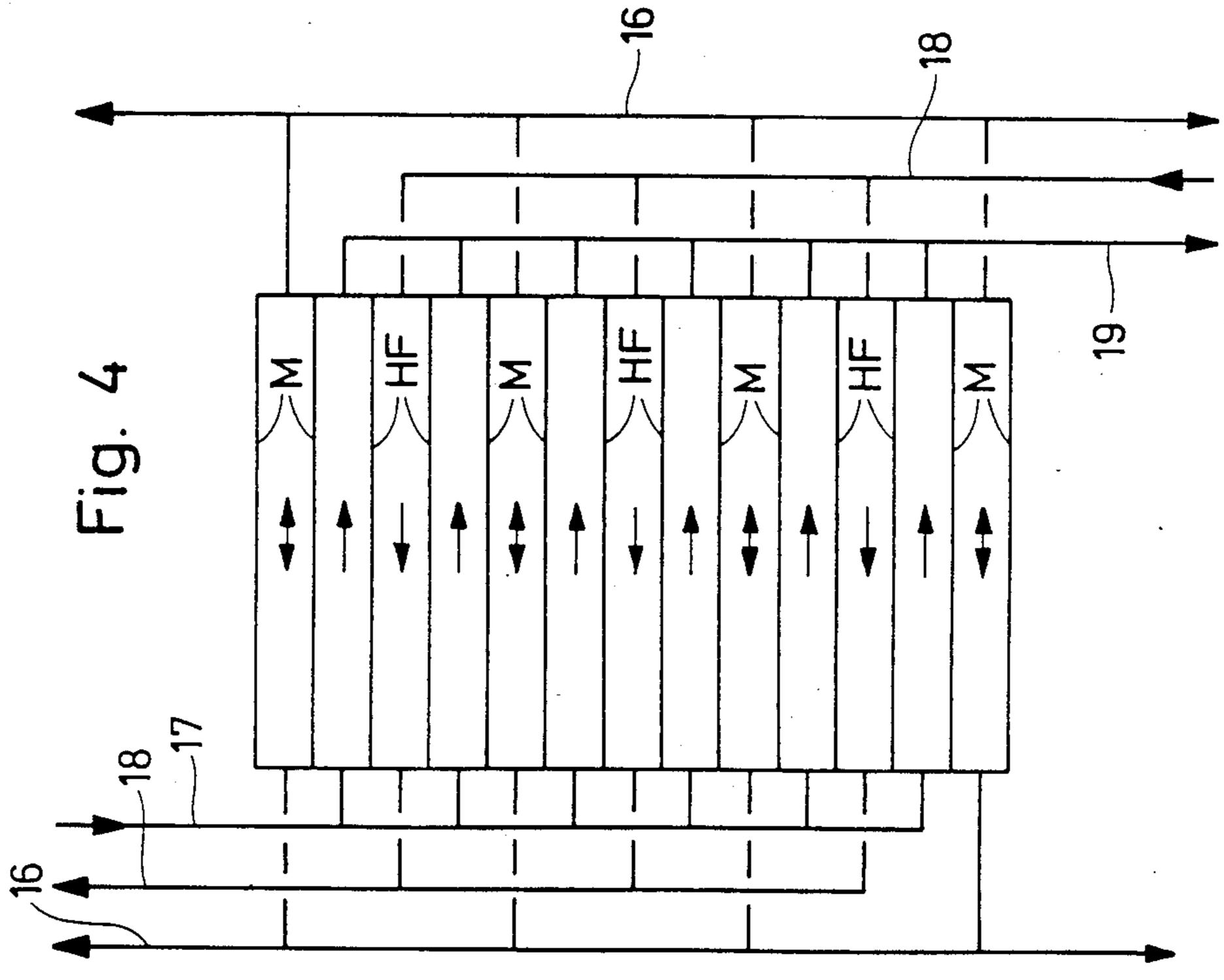
APPARATUS FOR THE SEPARATION OF SOLUTIONS BY PERVAPORATION
