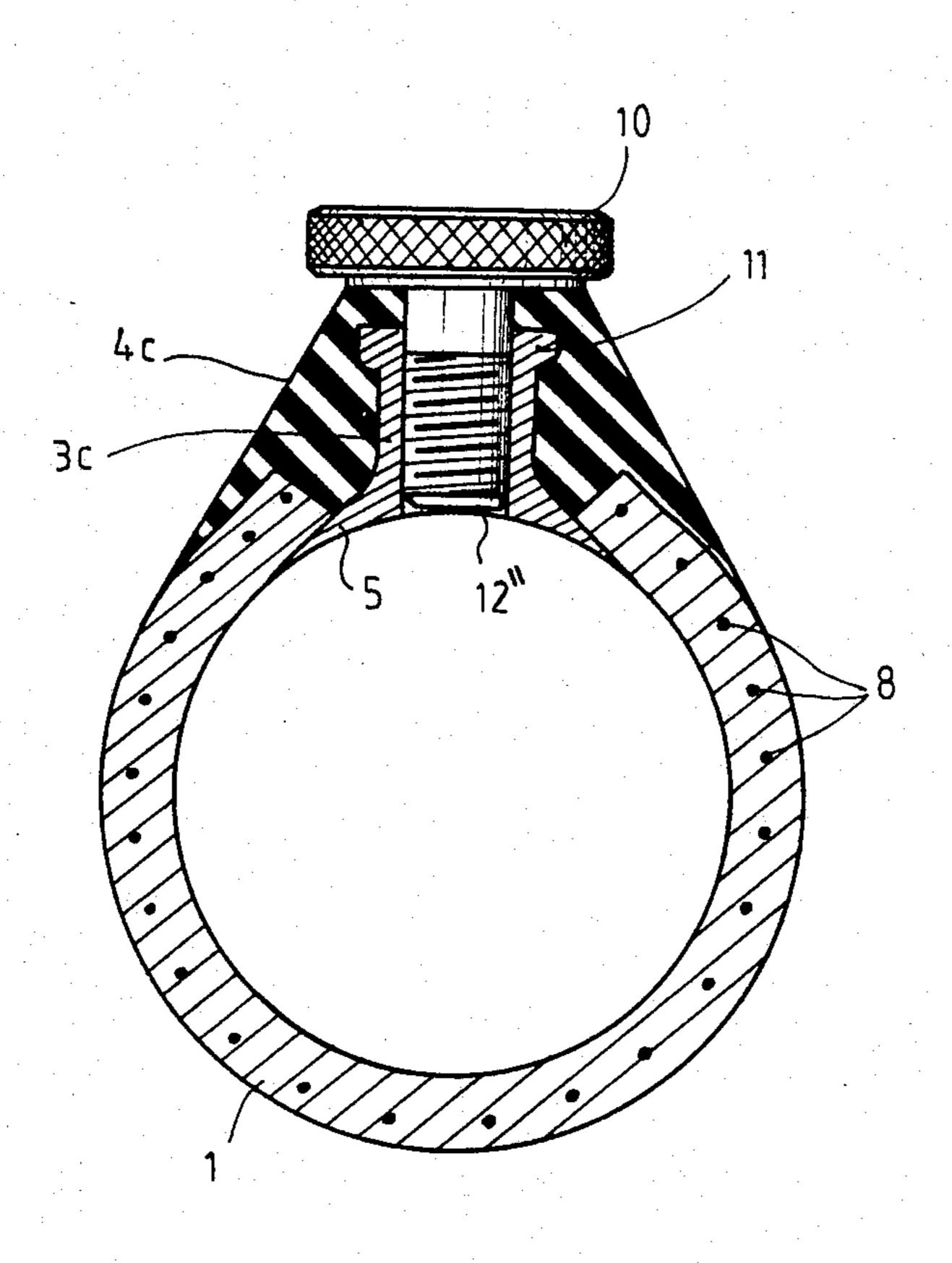
BYPASS CONNECTIONS OBTAINED BY MOLDING A COATING OF A JUNCTION MATERIAL AROUND A RIGID TUBULAR INSERT AND A PROCESS FOR MANUFACTURING SAME
