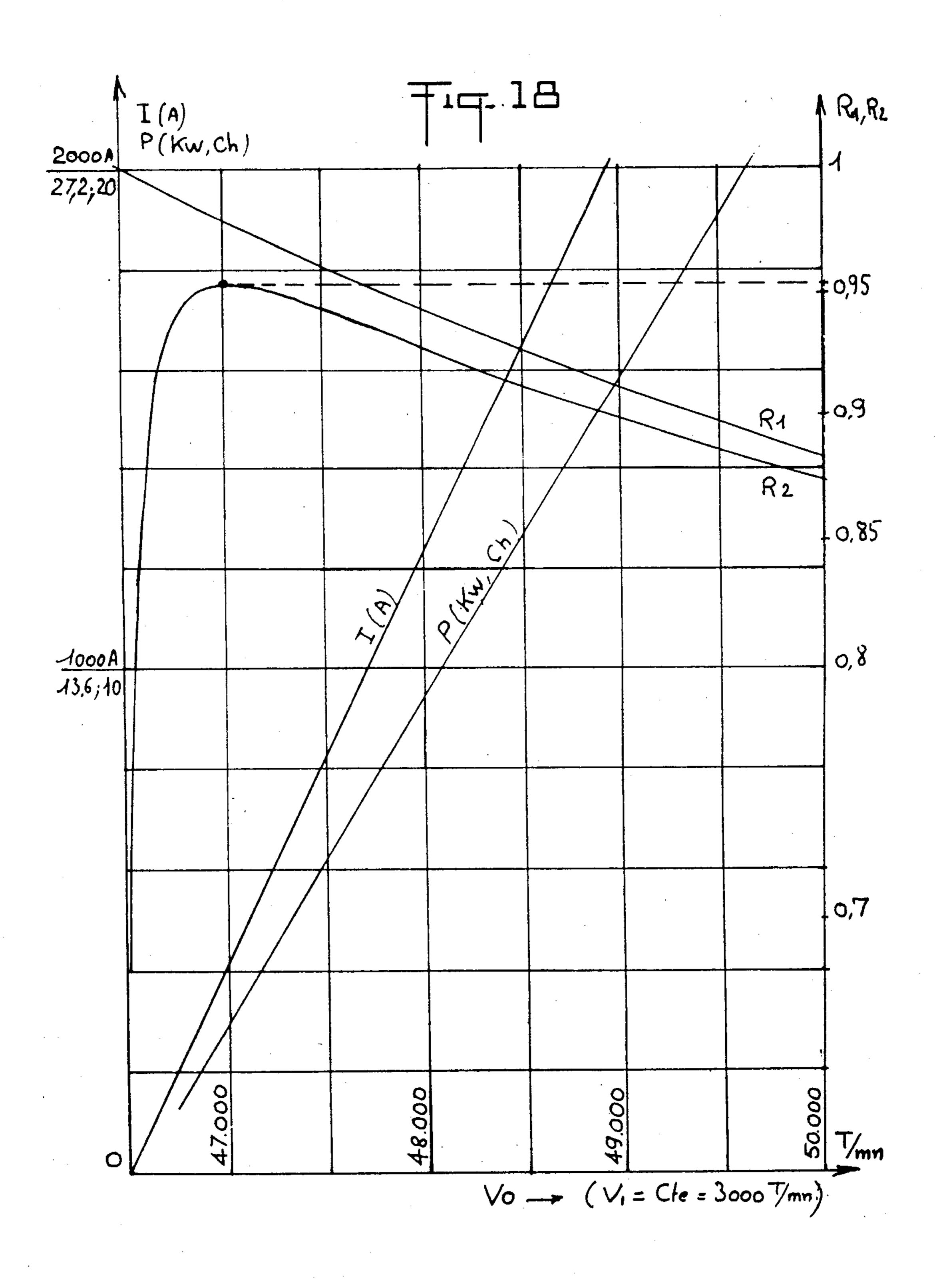
INDUCTION-TYPE PLANETARY REDUCING COUPLING FOR VERY HIGH SPEED ROTATING MACHINES
