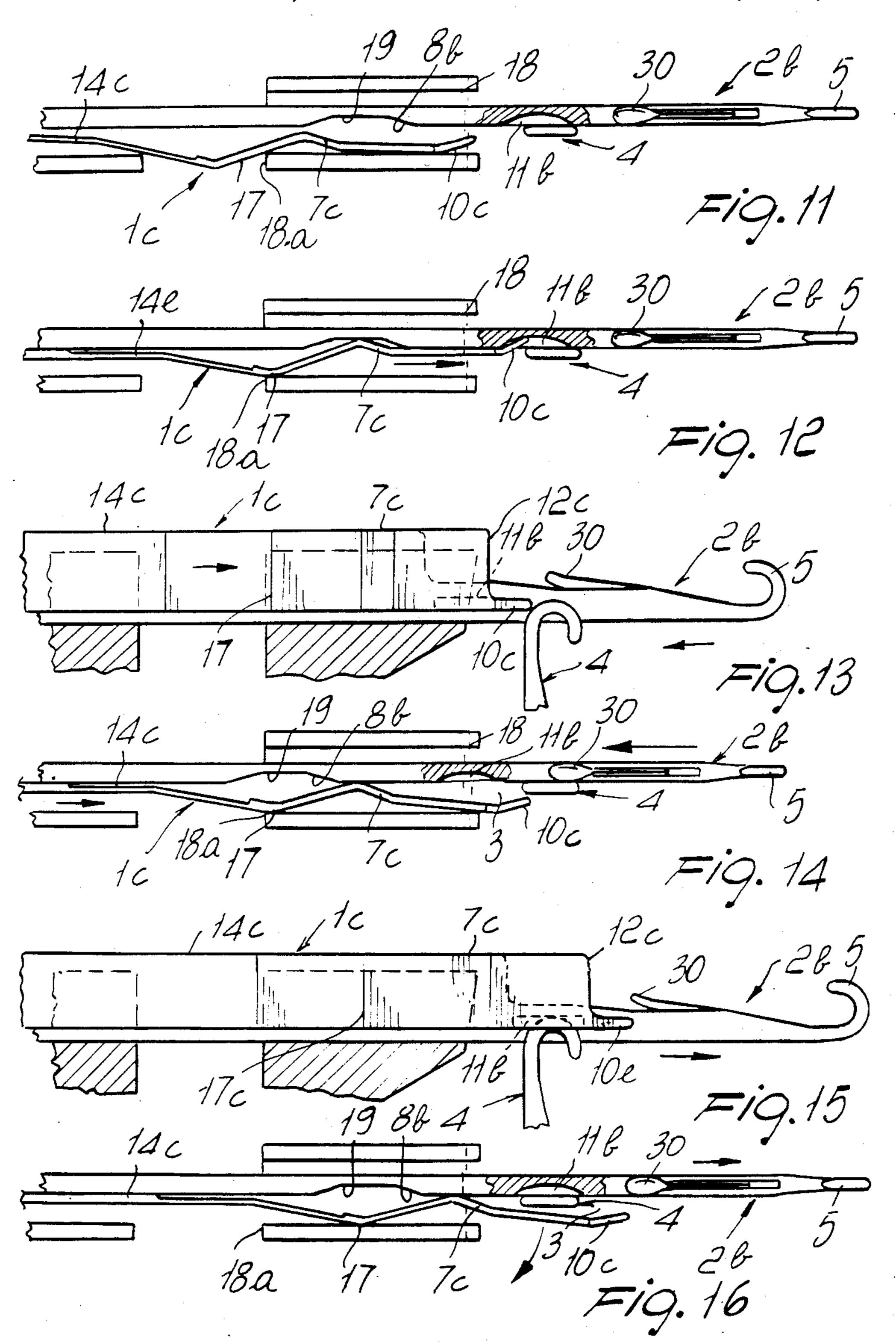
DEVICE FOR THE PASSING OF THE STITCH FROM A NEEDLE FOR THE FORMING OF PLAIN KNITTING TO A NEEDLE FOR THE FORMING OF PURL KNITTING AND VICE VERSA, IN A KNITTING MACHINE AND THE LIKE
