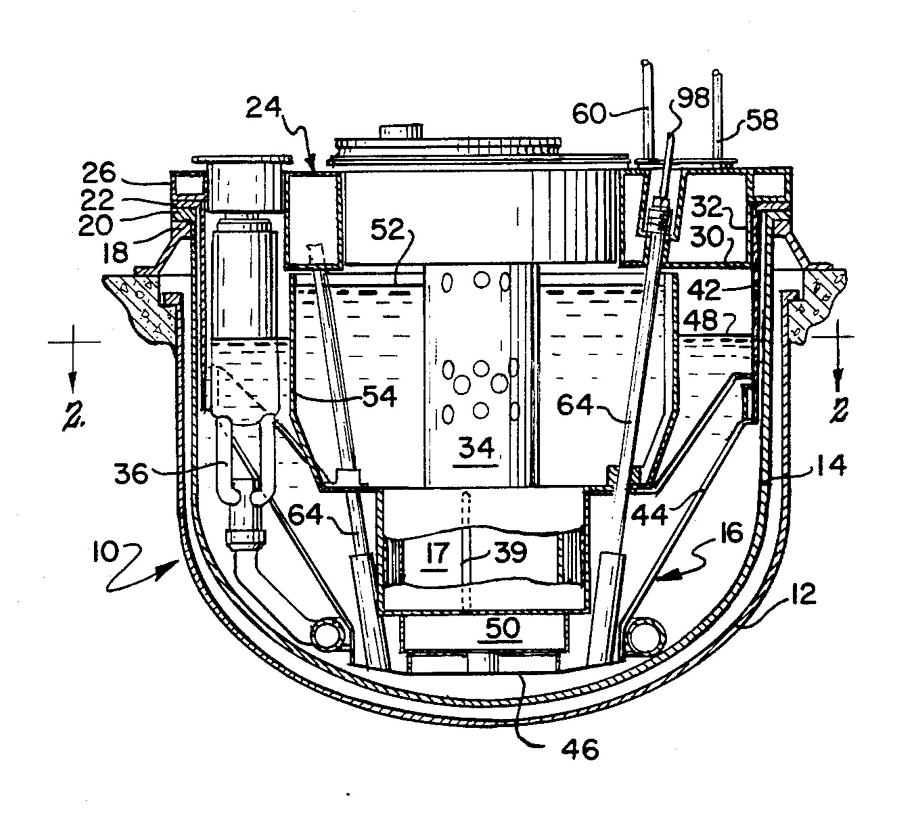
HANGING CORE SUPPORT SYSTEM FOR A **NUCLEAR REACTOR**
