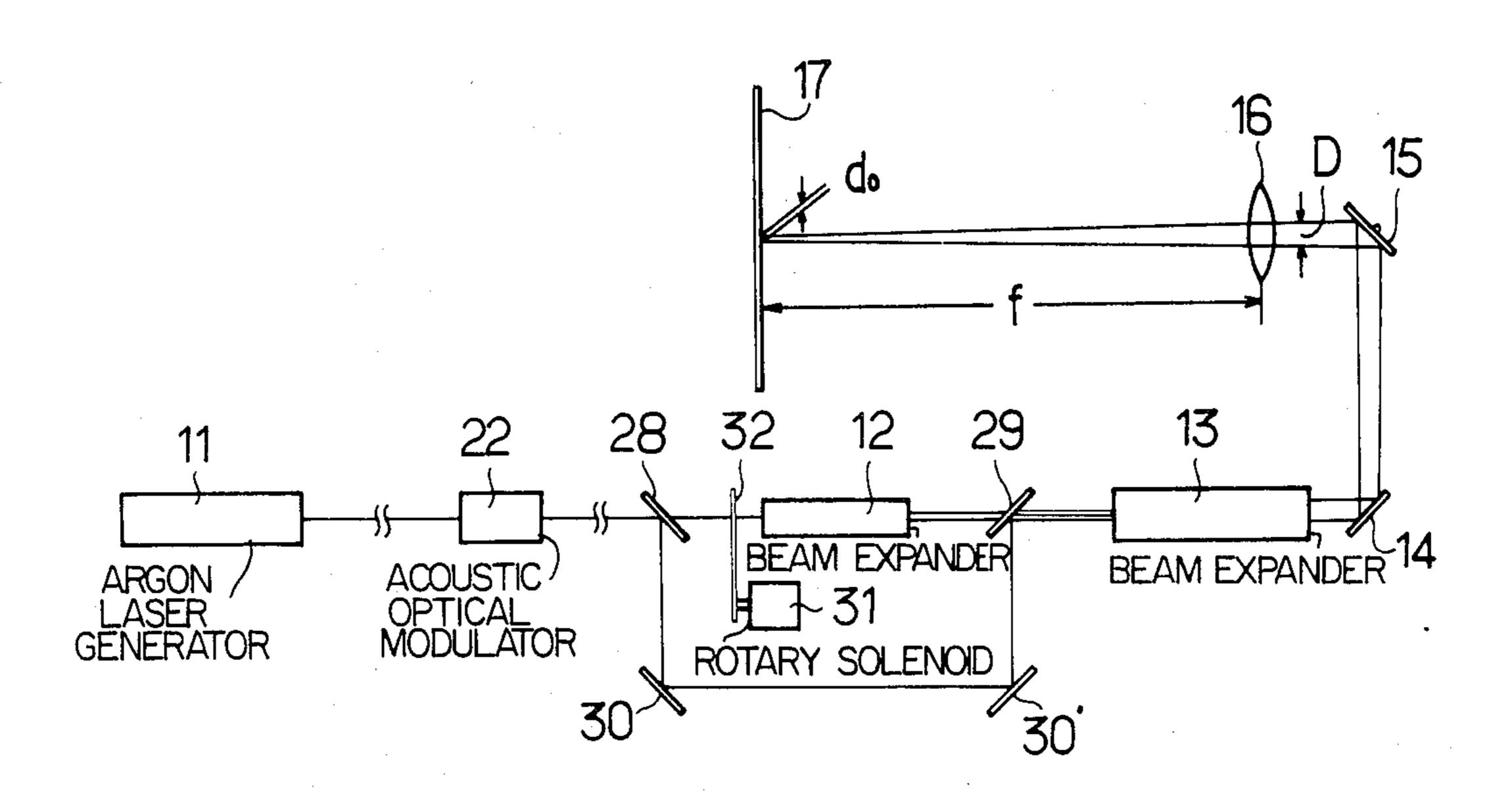
FIG. 2 is an explanatory view of the optical system with a diameter of a scanning beam changed in a switching manner.
