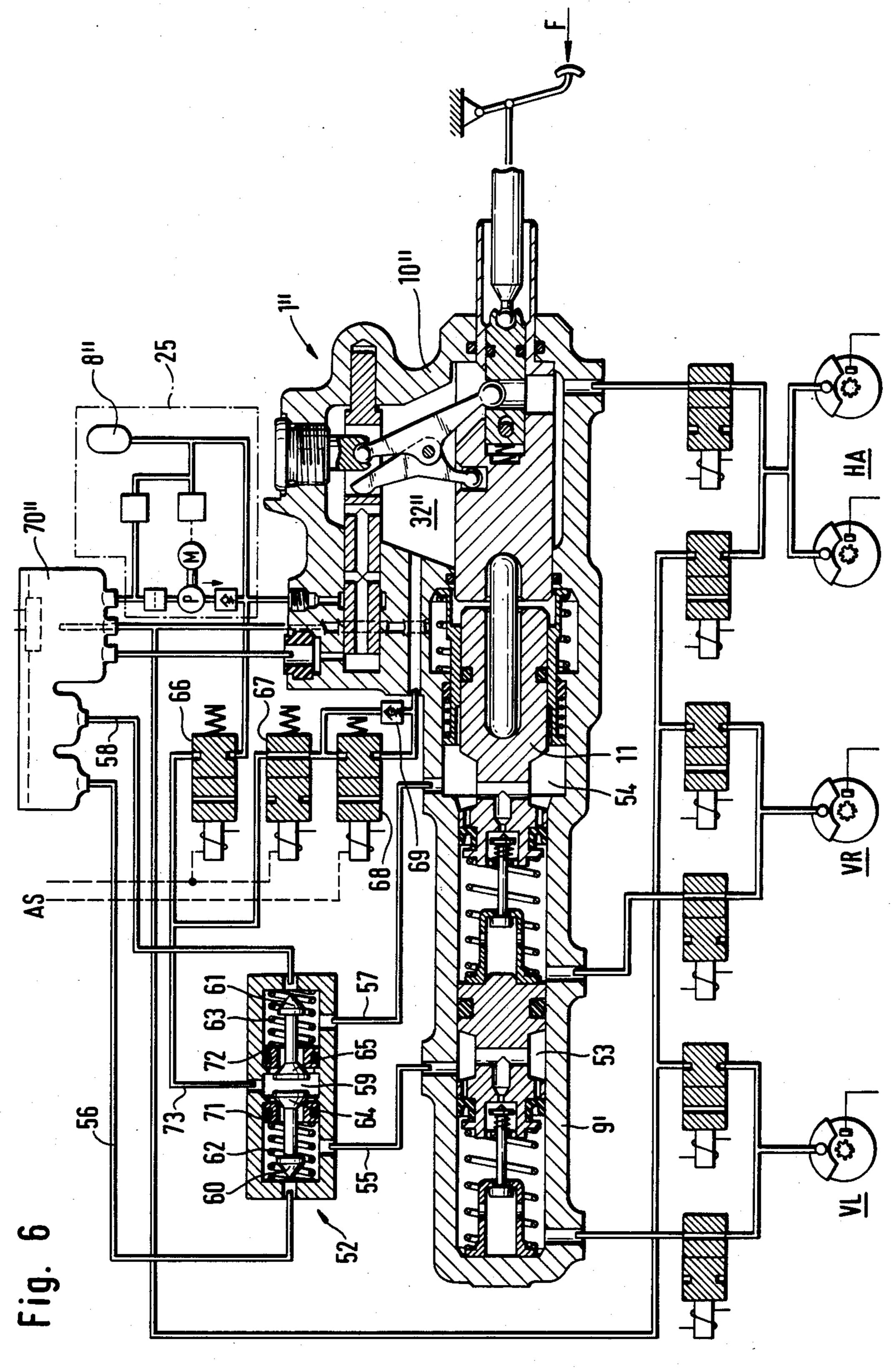
the master cylinder, according to a first embodiment of the present invention;
