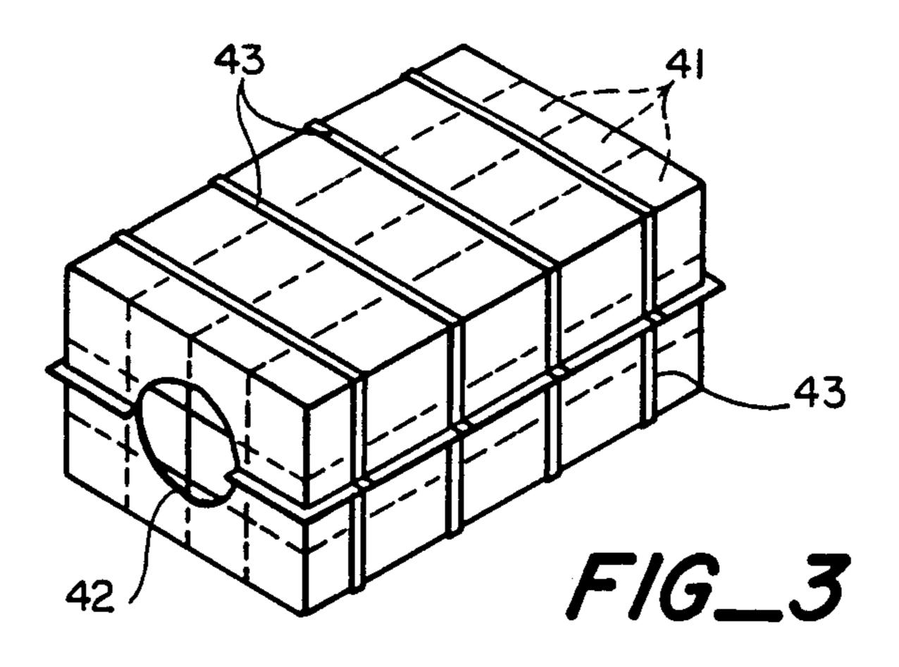
APPARATUS AND METHOD FOR WRAPPING PACKAGES WITH HEAT SHRINKABLE MATERIAL
