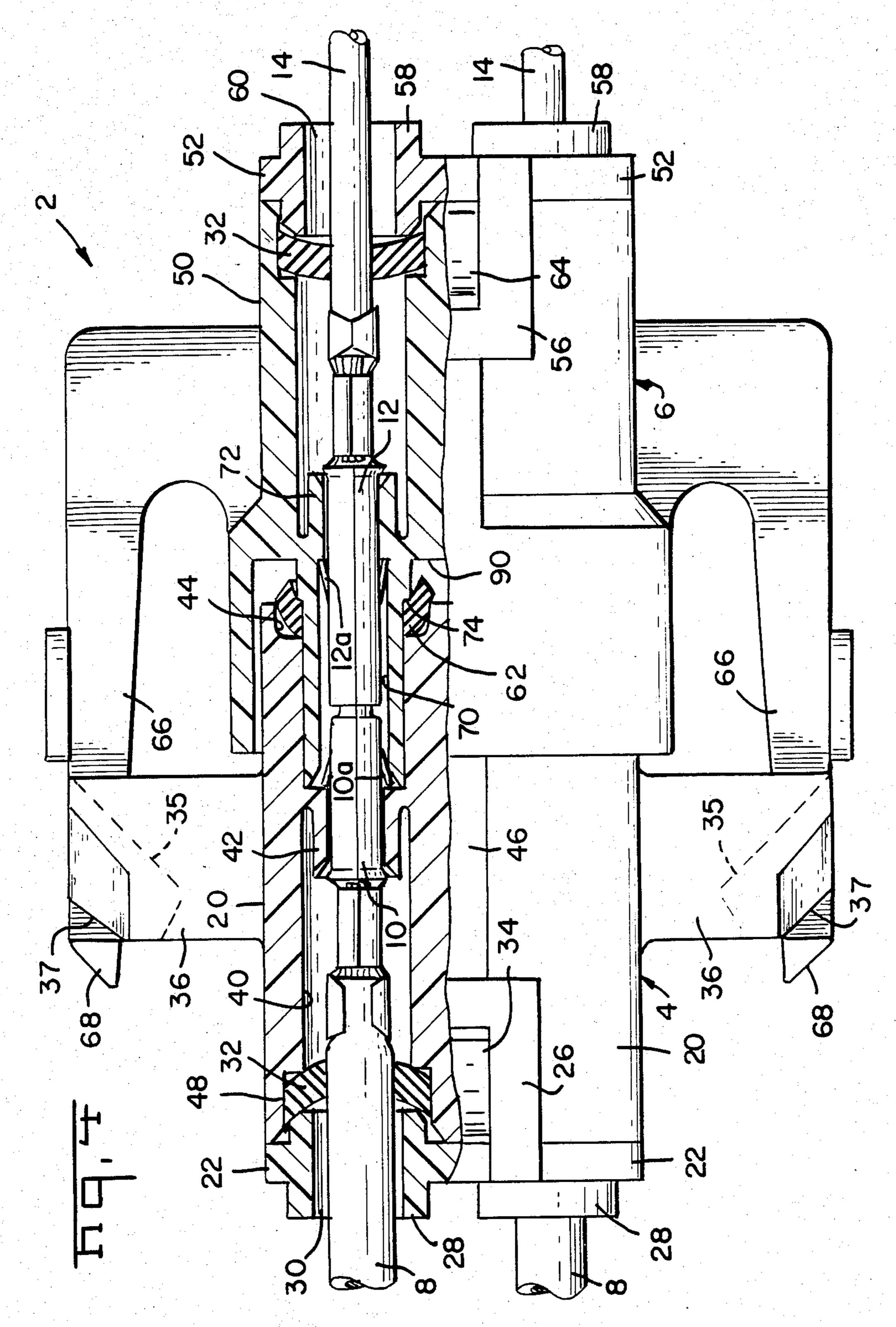
DETACHABLE SEALED MULTICONTACT ELECTRICAL CONNECTOR
