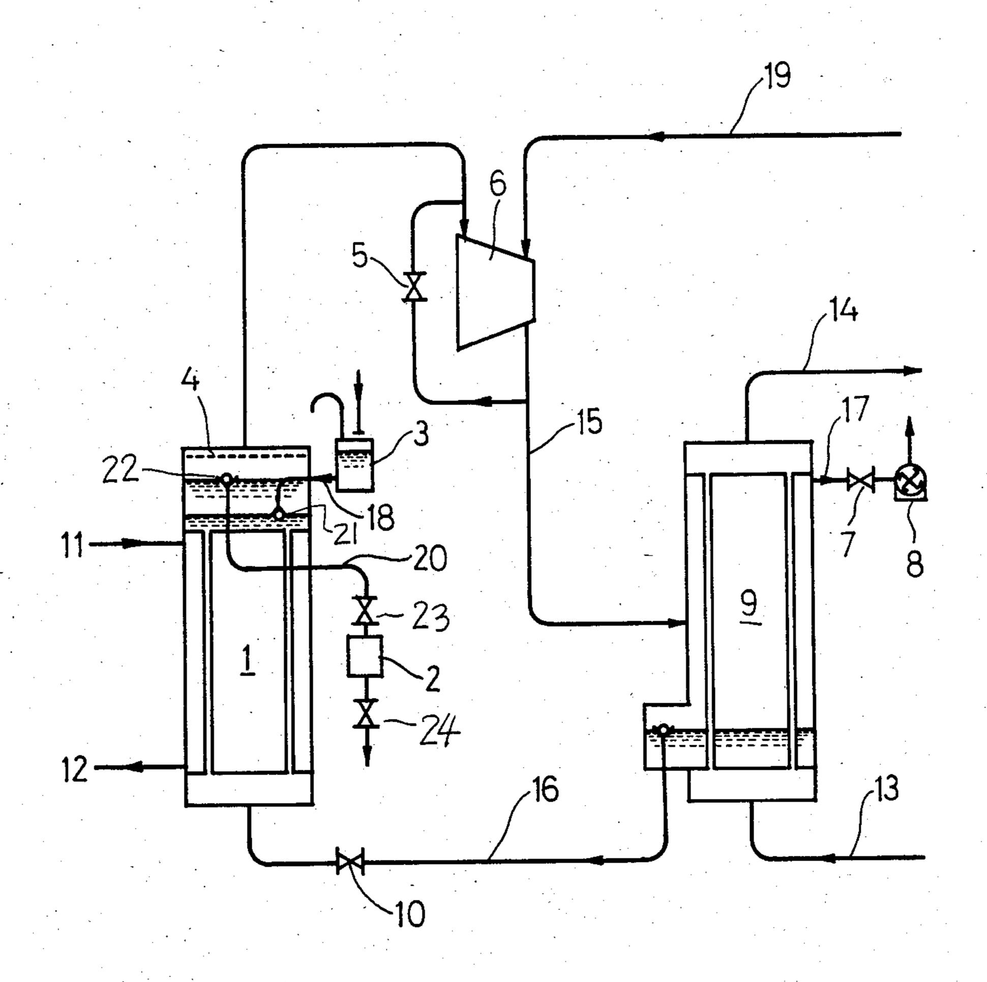
keep the water level in the evaporator and condenser constant.
