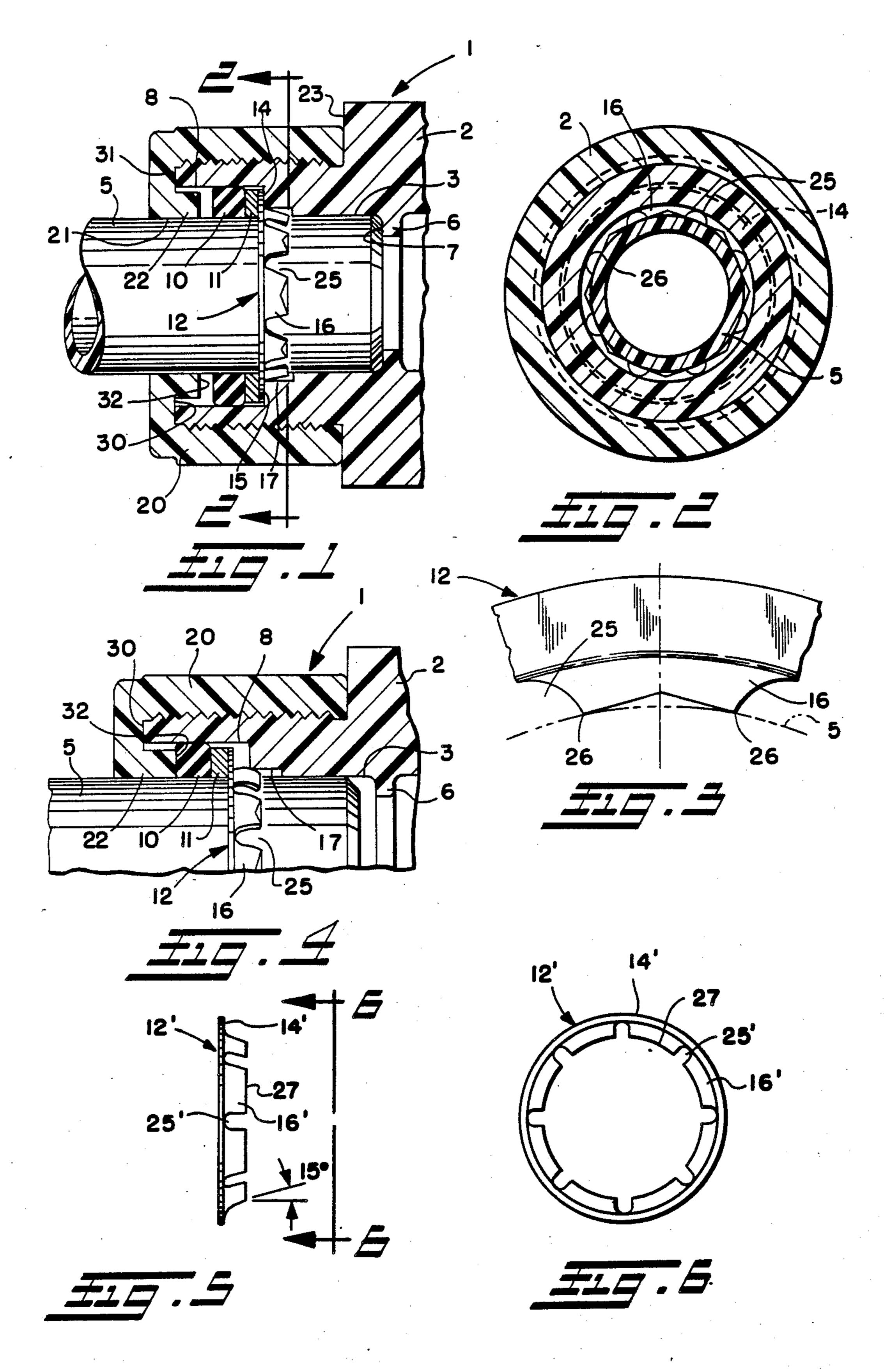
FIG. 2 is a transverse section through the tube coupling of FIG. 1, taken along the plane of the line 2—2
