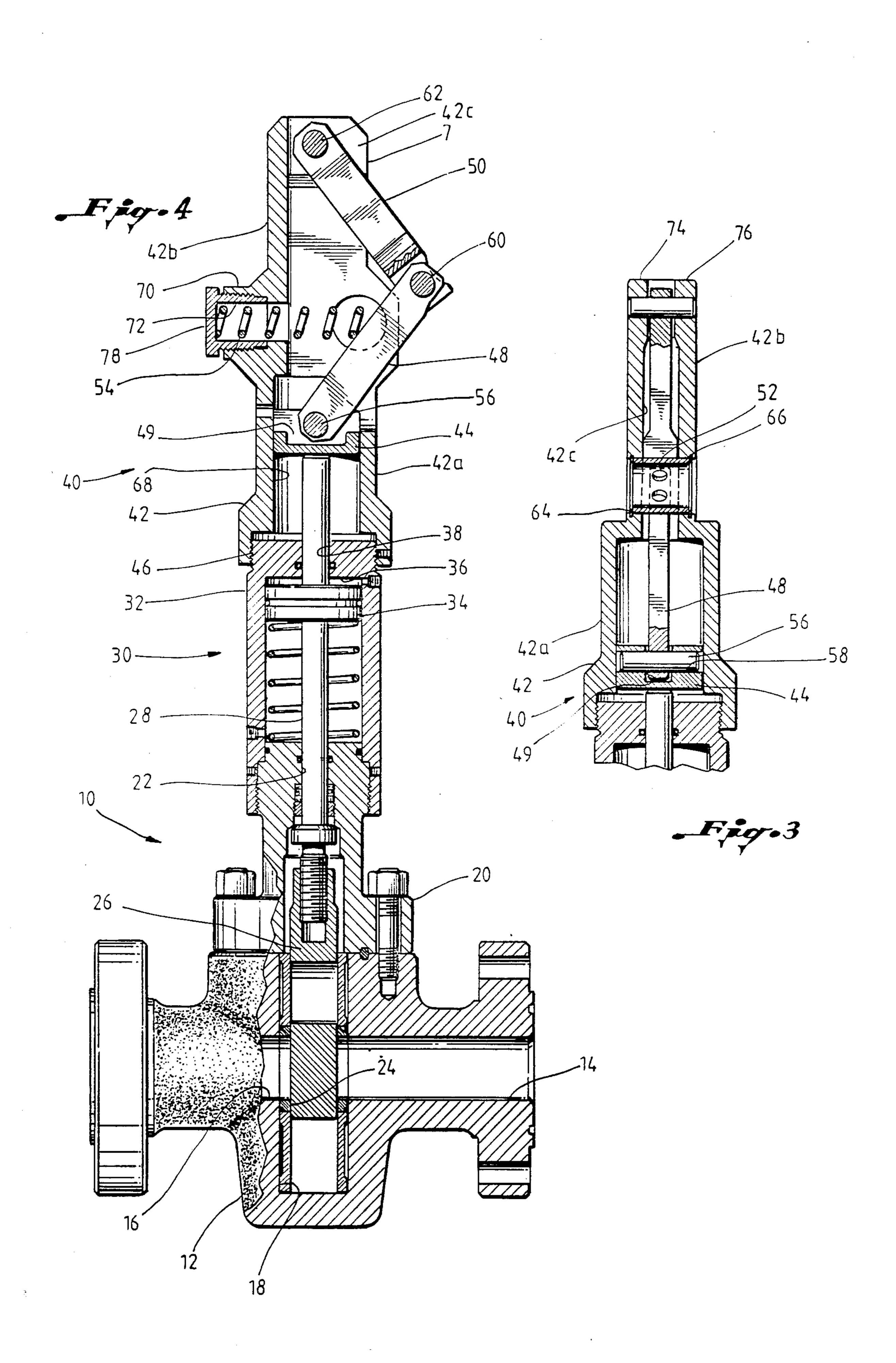
The present invention relates to an improved valve having a pressure responsive actuator which moves its 5 valve member and its attached stem between open and closed positions. Such valves are commonly used in workovers on oil and gas wells and they are installed and actuated to their open position when work is to proceed on the well. The valve is intended to be heat 10 closing. responsive so that if a fire occurs, the valve will close to
