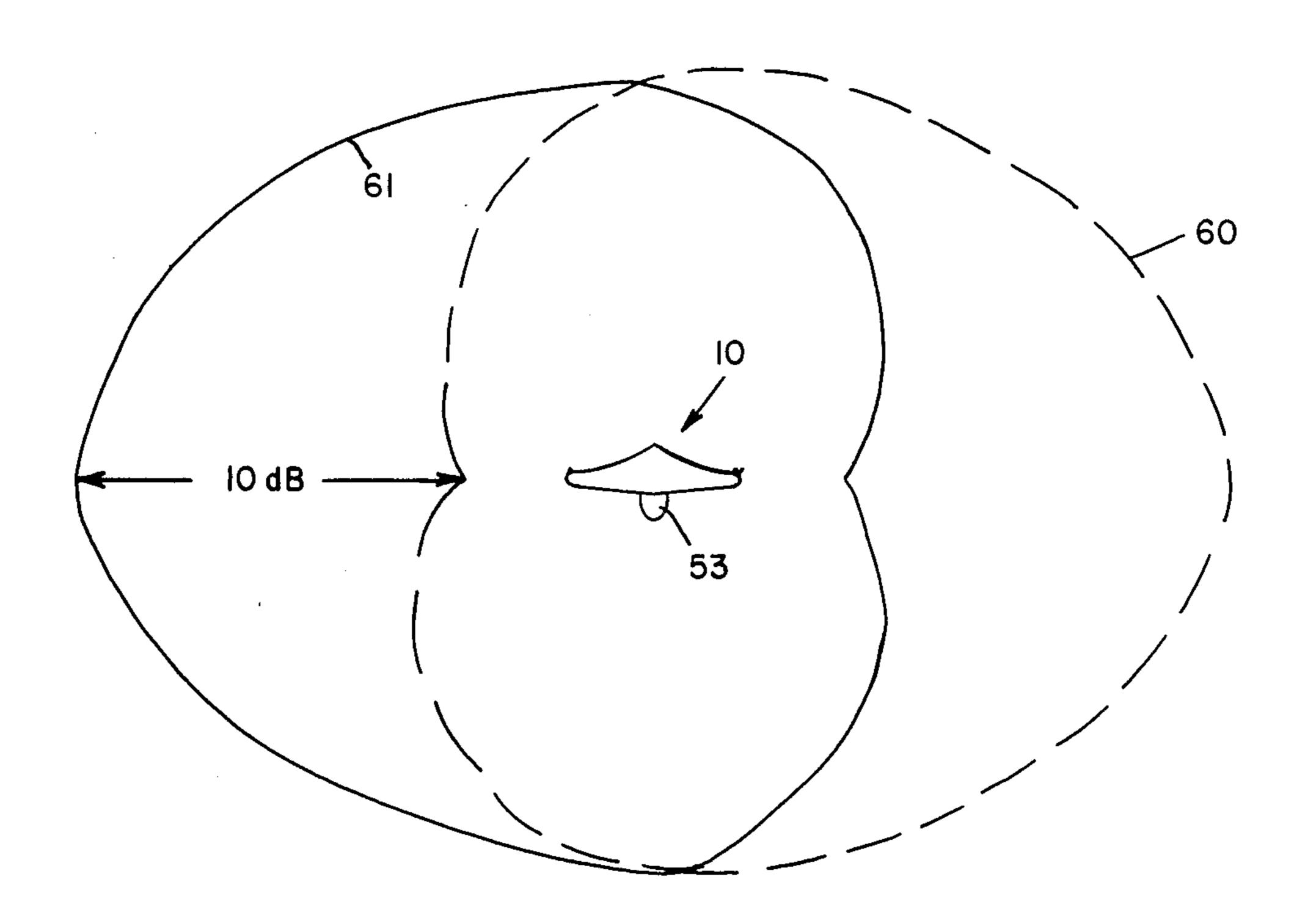
leg elements to enhance the reception for the directional antenna section.
