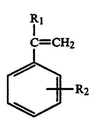
10 wherein R<sub>1</sub> represents a hydrogen, or an alkyl group having 1 to 6 carbon atoms, and R<sub>2</sub> represents a hydrogen atom, a halogen atom, or an alkyl group having 1 to 6 carbon atoms.
