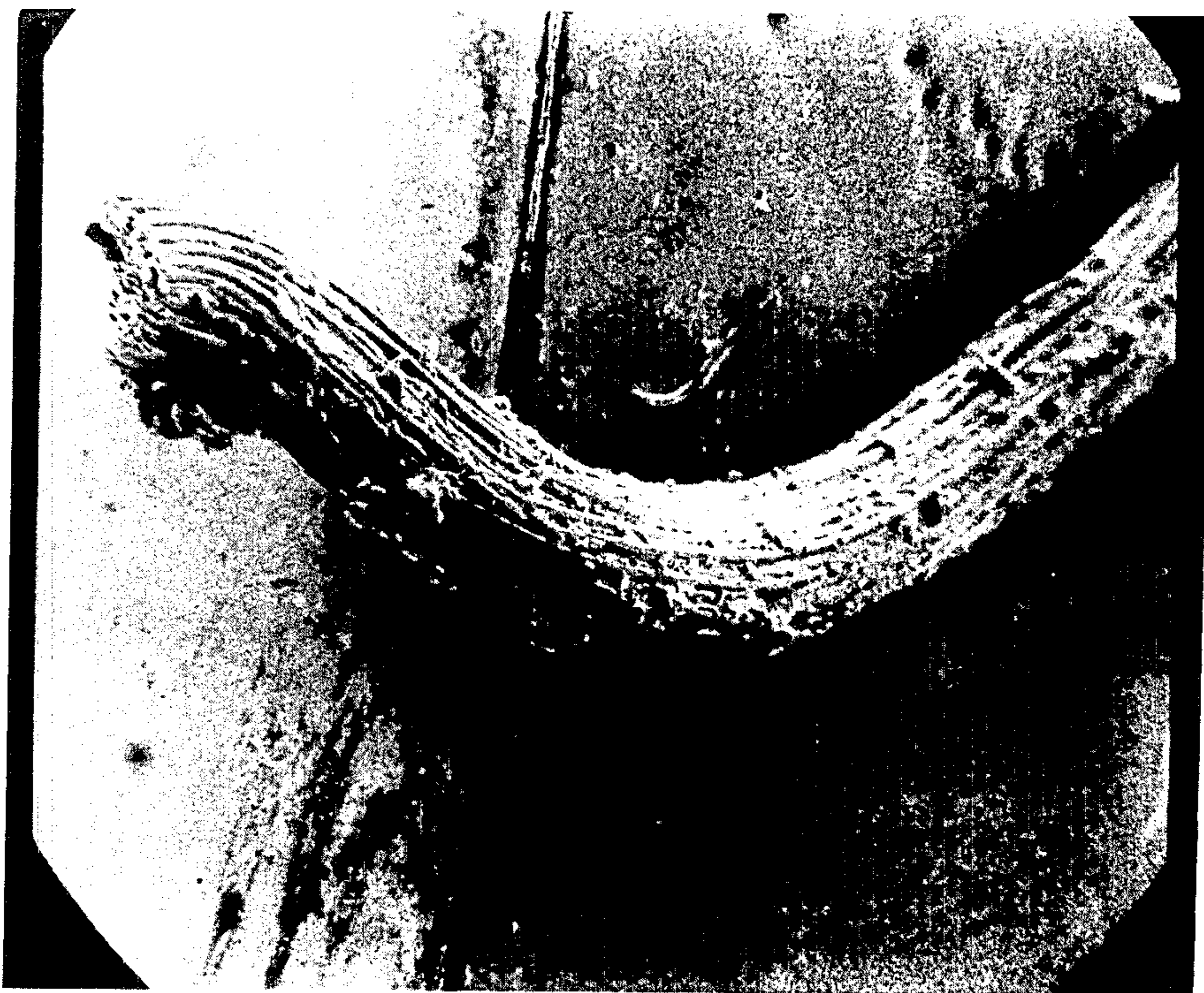
FIGURE 5a - PULLED-OUT FIBER
