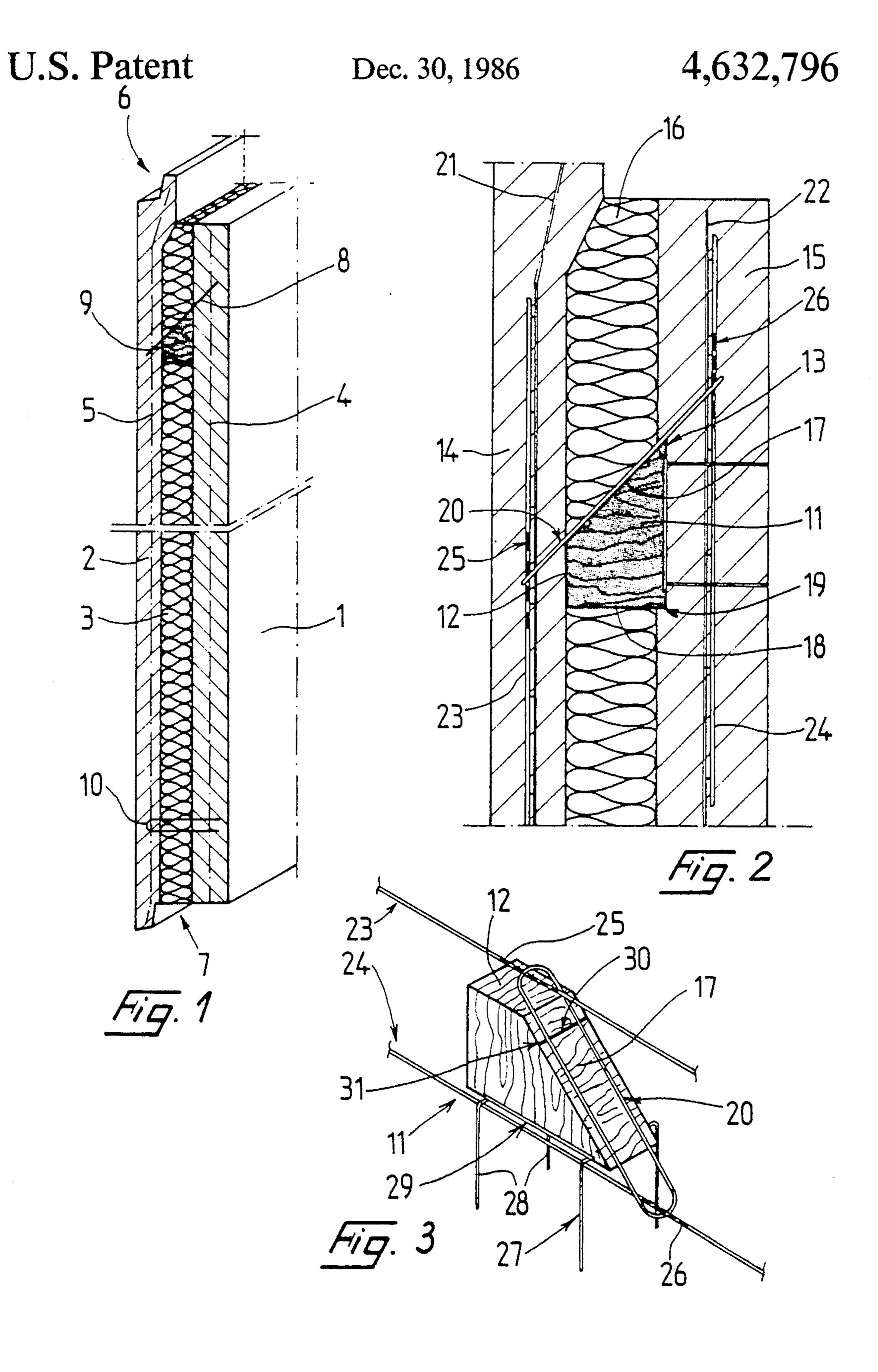
METHOD OF MANUFACTURING A SANDWICH WALL PANEL BY MOLDING
