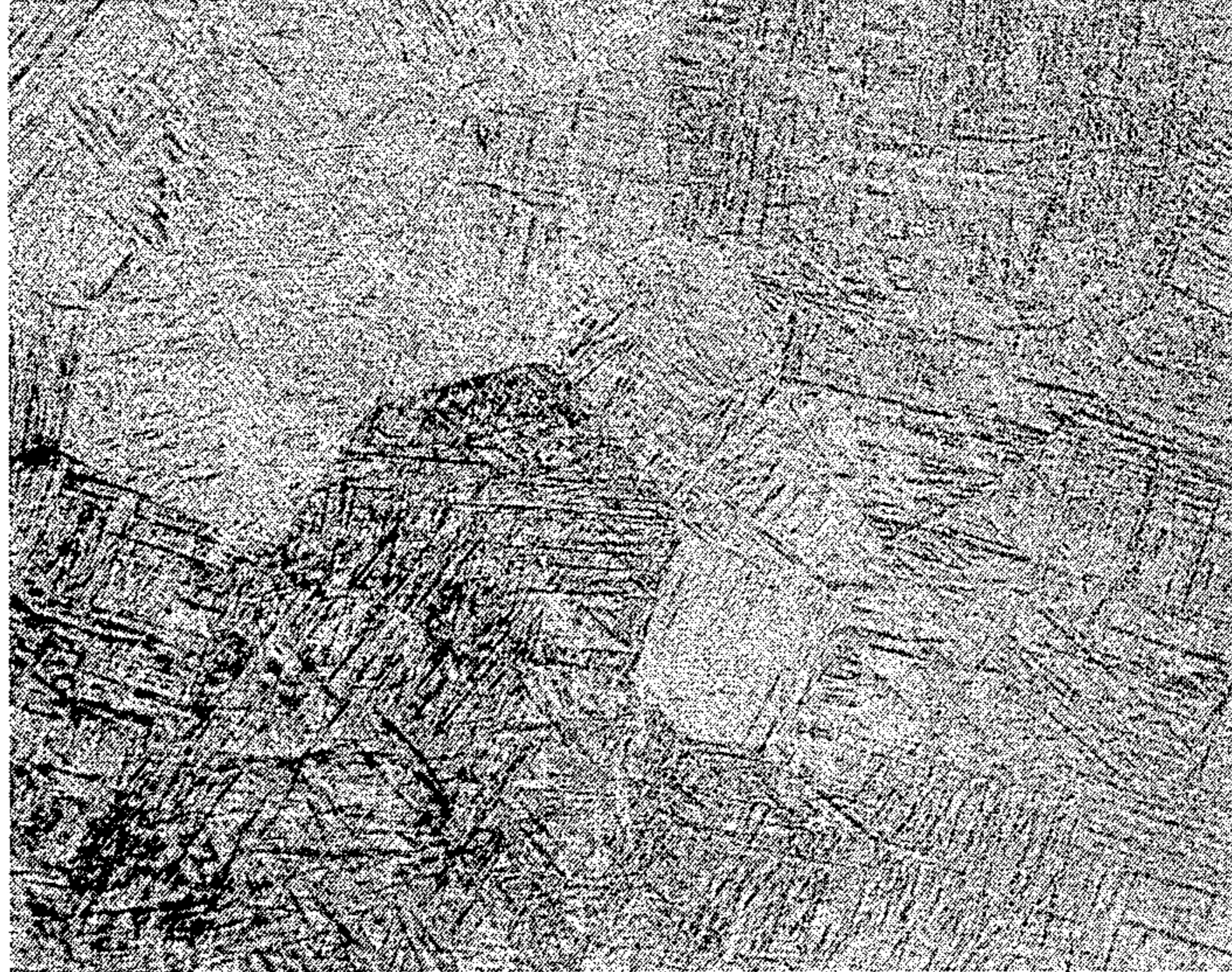
FIG. 4 FAN BLADE HEAT TREATED ABOVE BETA TRANSUS TEMPERATURE.
