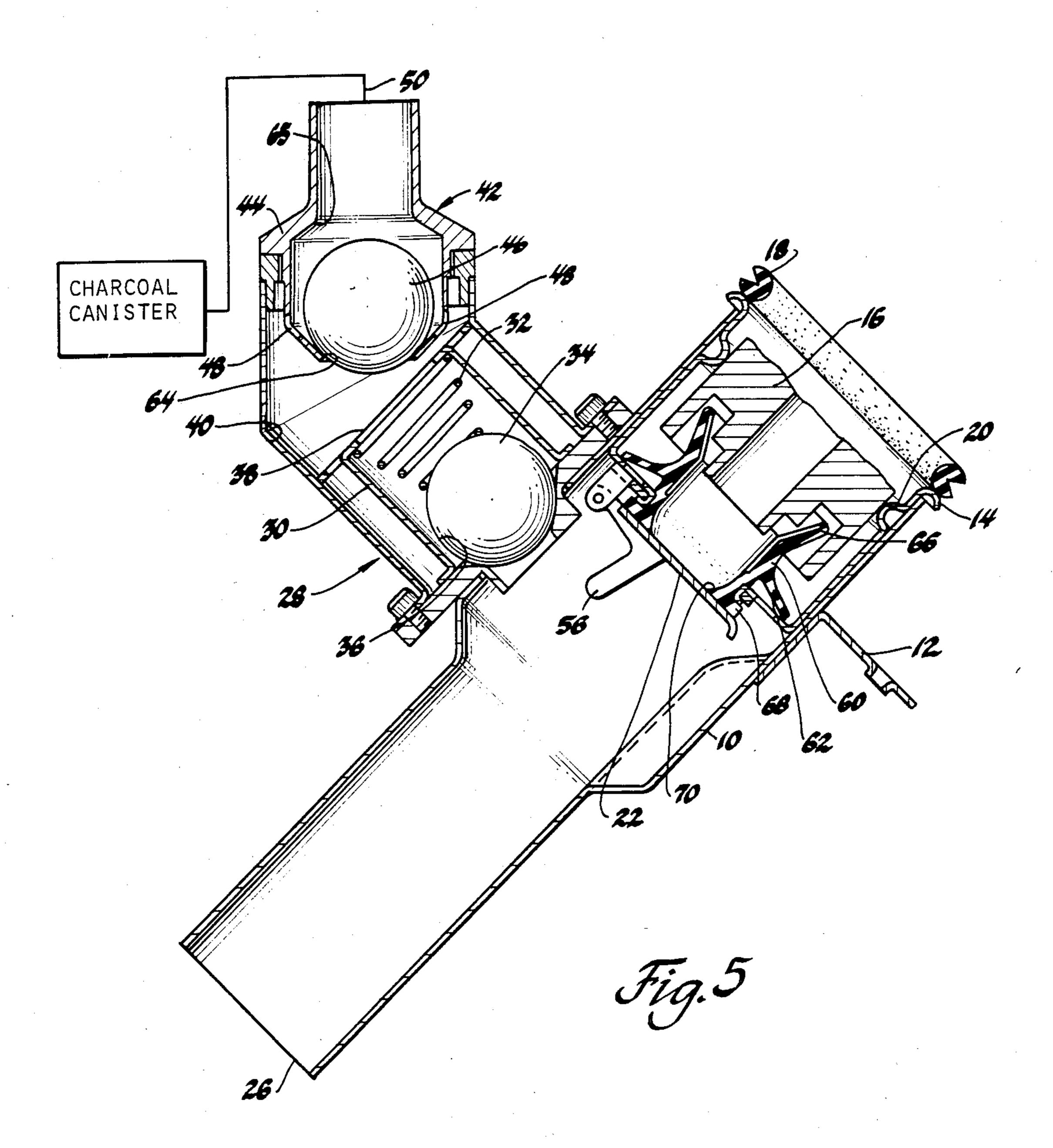
of an extension 25 on the fuel cap 16 to provide a seal arrangement when the cap is installed.
