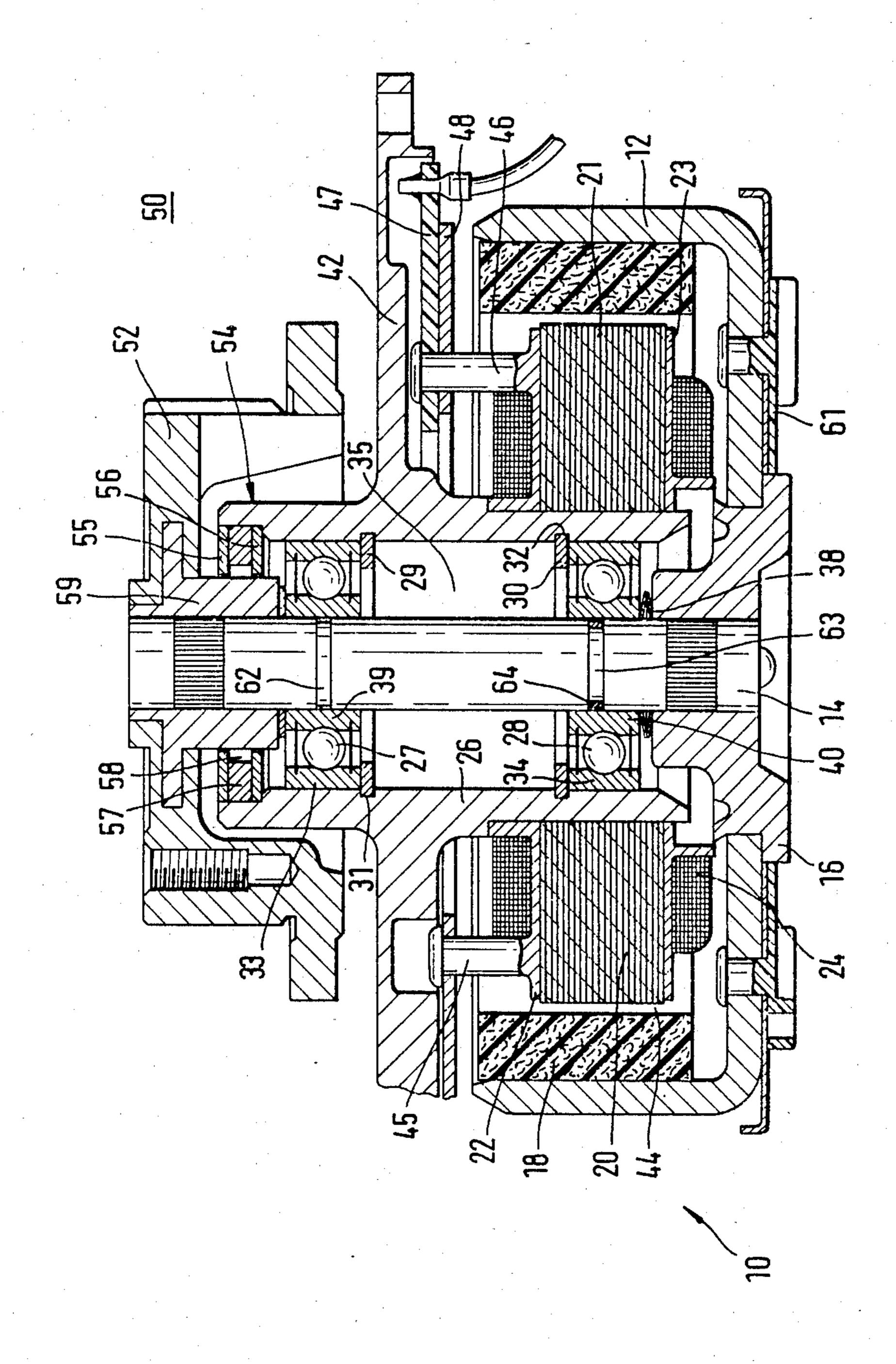
radial displacements of the motor rotation axis, e.g. by vibrations in the clearance between the bearing inner
