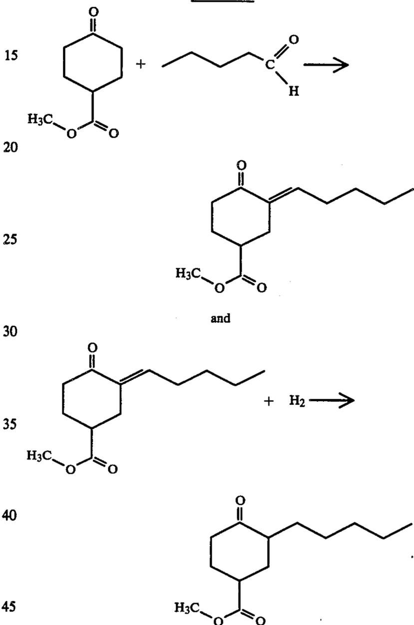
Into a 3-liter reaction vessel equipped with stirrer, thermometer, reflux condenser and hydrogen chloride inlet is placed a mixture of 400 ml toluene and 290 grams of the ketoester having the structure:
