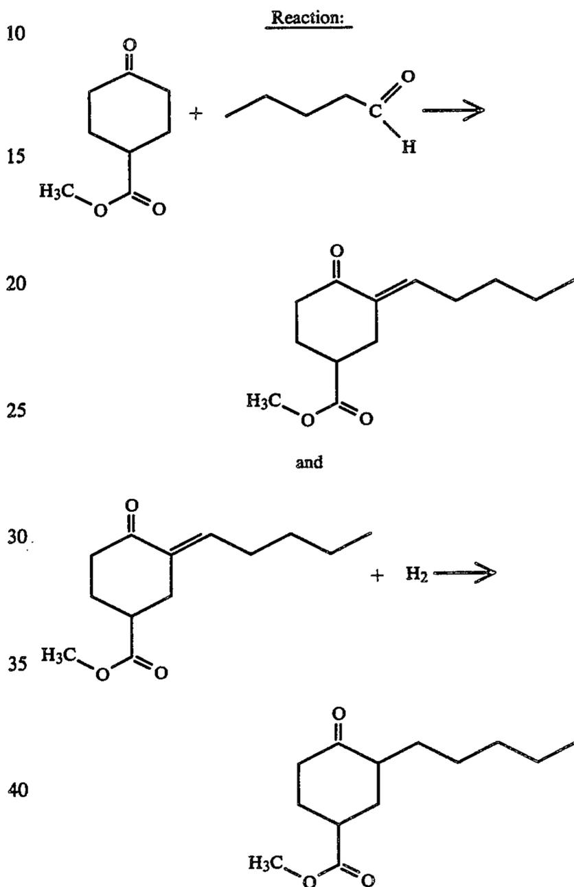
Into a 300 cc reaction vessel equipped with stirrer, thermometer, reflux condenser and inlet hydrogen chloride gas tube is placed a mixture of 40 ml toluene and 15.6 grams of keto ester having the structure:
