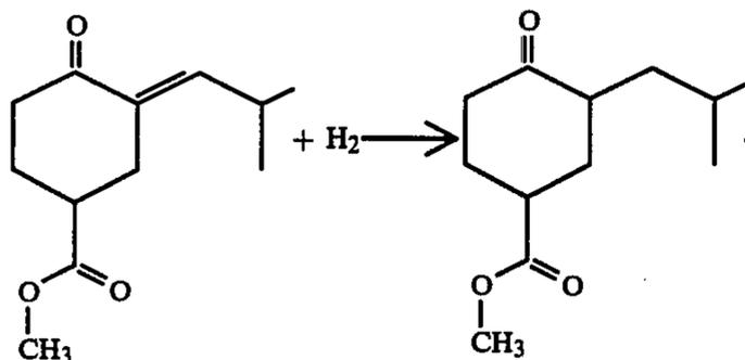
Into a 300 cc reaction vessel equipped with stirrer, thermometer, reflux condenser, cooling coils and hydrogen chloride inlet tube is placed a mixture of 50 ml toluene and 15.8 grams of the ketoester having the structure:
