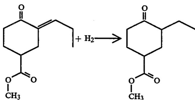
Into a 300 cc reaction flask equipped with stirrer thermometer, reflux condenser cooling bath and hydrogen chloride inlet tube is placed a mixture of 48 ml toluene and 15.8 grams of ketoester having the structure:
