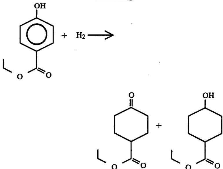
Into a 1-liter magnetically stirred autoclave is placed 489 grams of ethyl-p-hydroxybenzoate having the structure:
